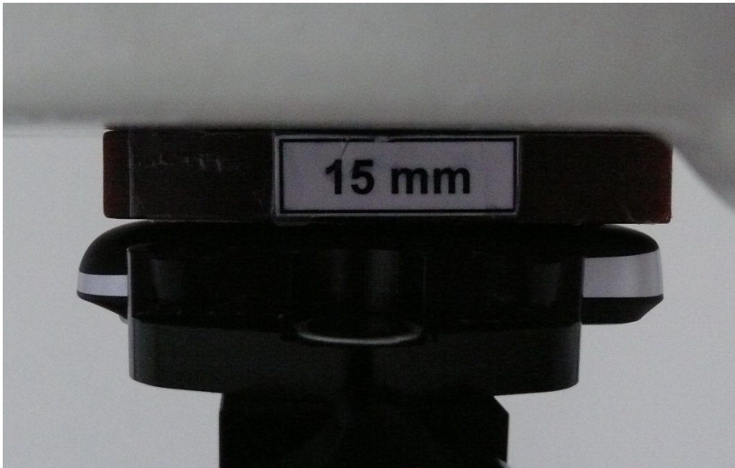
Picture 13: Body, The EUT display towards ground, the distance from handset to the bottom of the Phantom is 15mm (The spacer was removed during testing)
