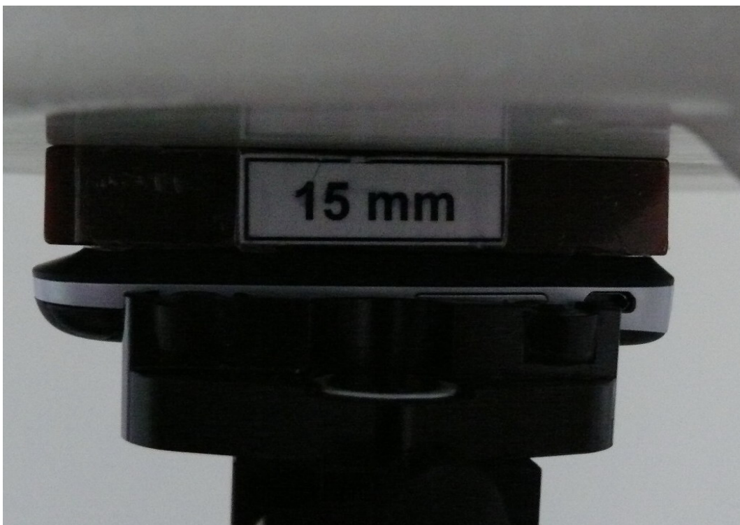
Picture 14: Body, The EUT display towards phantom, the distance from handset to the bottom of the Phantom is 15mm (The spacer was removed during testing)
