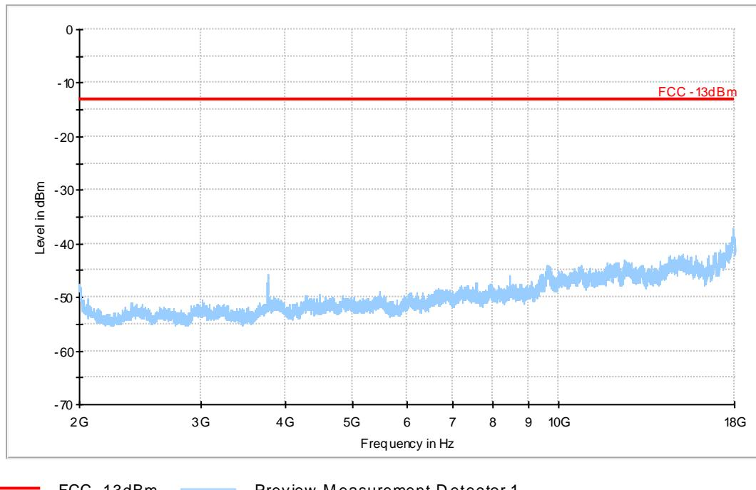
**A.2.3.6 RADIATED SPURIOUS EMISSIONS-Channel 9538: 2GHz – 18GHz**
