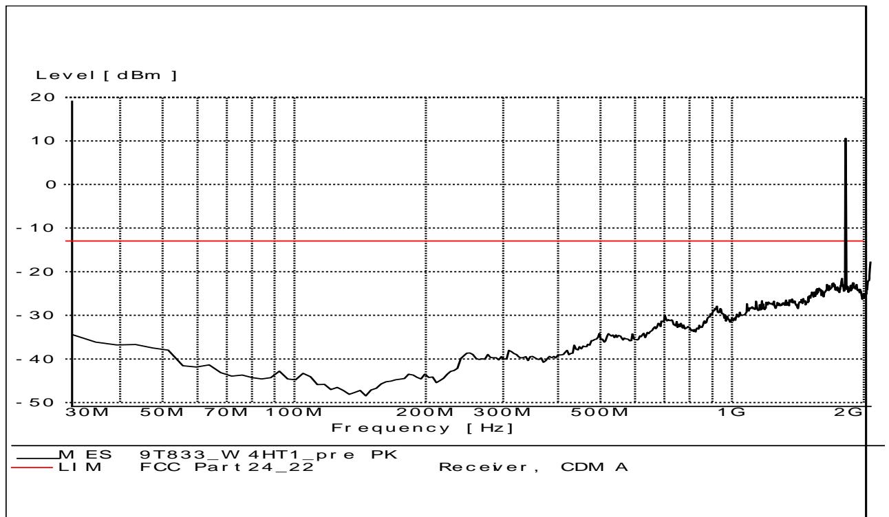
**A.2.3.14 RADIATED SPURIOUS EMISSIONS-Channel 1312: 2GHz – 18GHz****Radiated spurious emission limit :-13dBm.**
