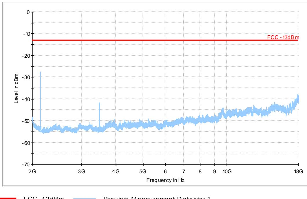
**A.2.3.16 RADIATED SPURIOUS EMISSIONS-Channel 1513: 2GHz – 18GHz****Radiated spurious emission limit :-13dBm.**
