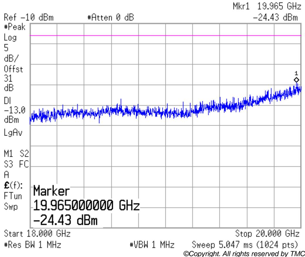
**WCDMA Band IV****A.2.3.11 RADIATED SPURIOUS EMISSIONS-Channel 1312: 30MHz –2GHz**
