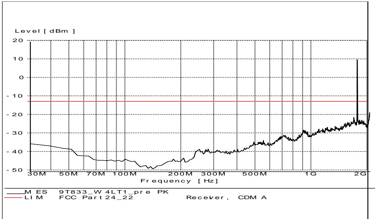
**A.2.3.12 RADIATED SPURIOUS EMISSIONS-Channel 1450: 30MHz – 2GHz**
