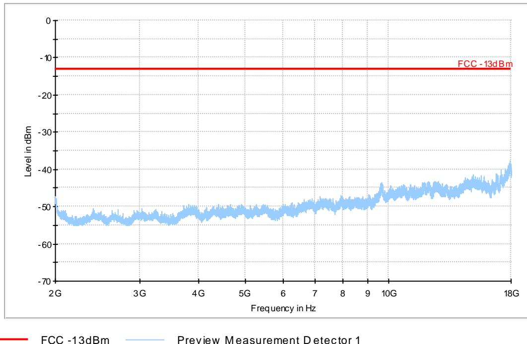
**A.2.3.14 RADIATED SPURIOUS EMISSIONS-Channel 810: 2GHz – 18GHz**
