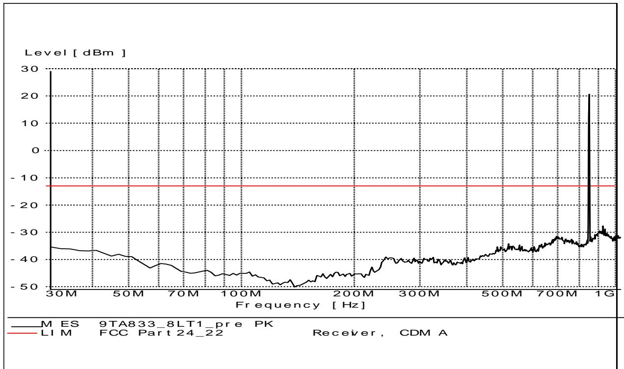
**A.2.3.2 RADIATED SPURIOUS EMISSIONS-Channel 190: 30MHz – 1GHz****Radiated spurious emission limit :-13dBm.****NOTE: peak above the limit line is the Carrier frequency @ ch-190**
