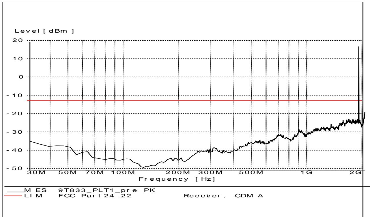
**A.2.3.10 RADIATED SPURIOUS EMISSIONS-Channel 661: 30MHz – 2GHz****Radiated spurious emission limit :-13dBm.****NOTE: peak above the limit line is the Carrier frequency @ ch-661**
