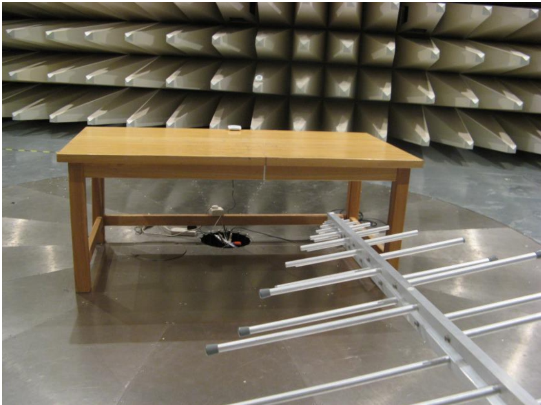
Part15C radiated emission
