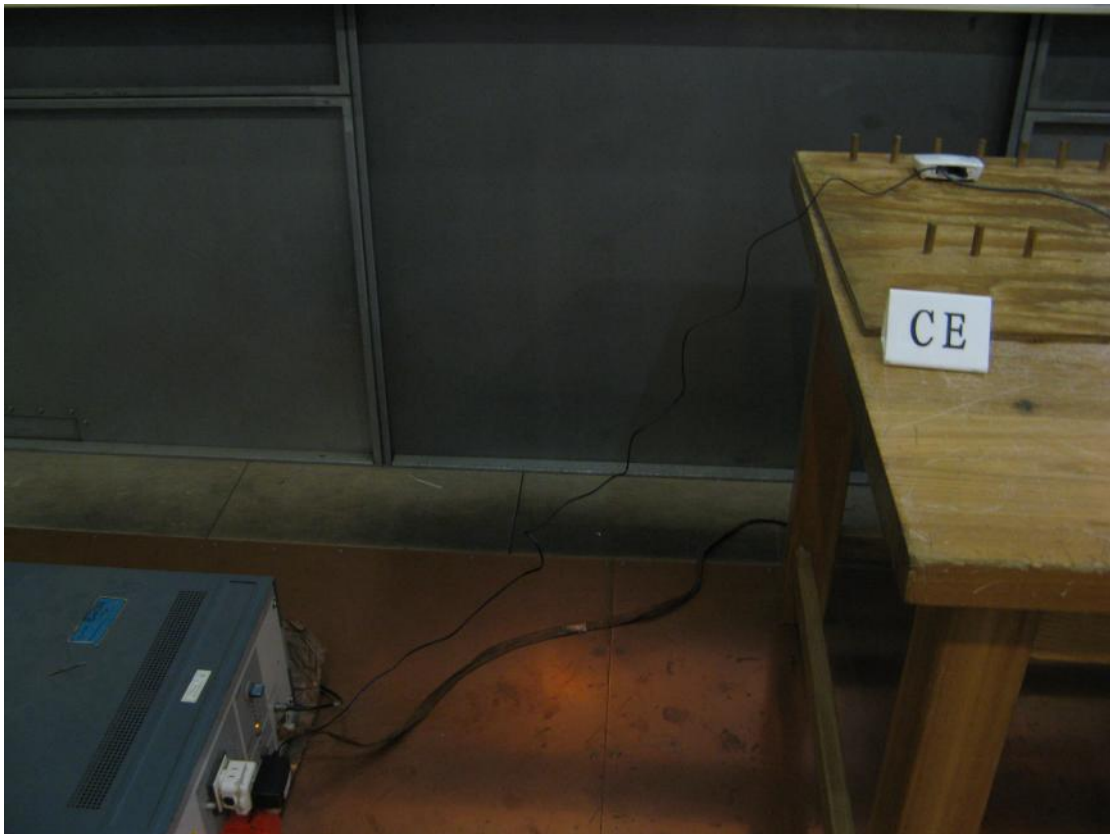
Part15C conducted emission
