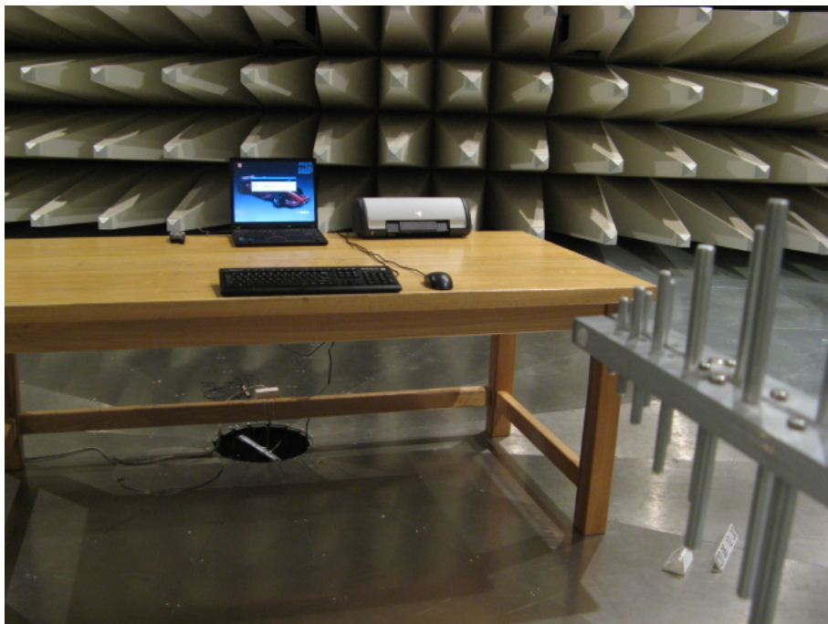
Pic C-4 Radiated Spurious Emission (USB Mode)
