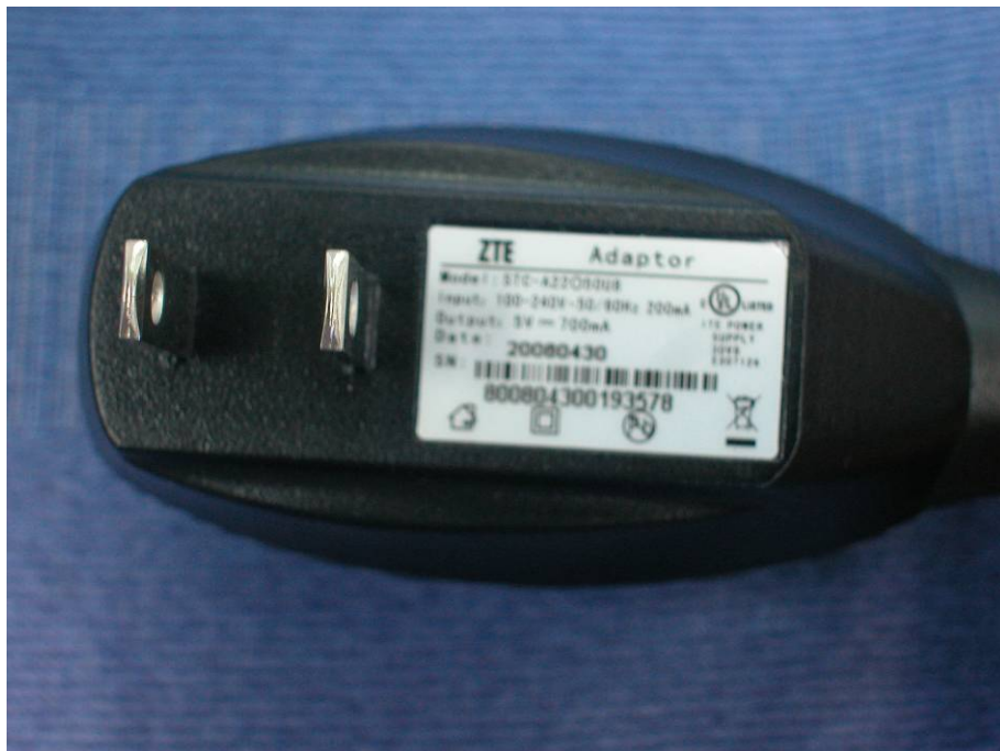
Label of Charger (AC/DC Adapter)
