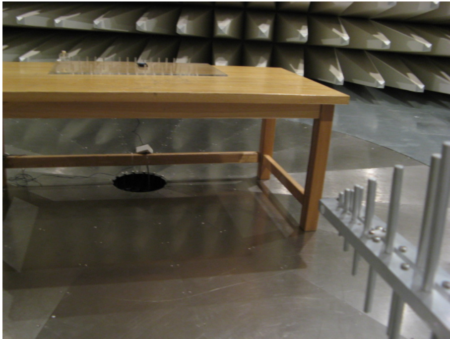
Pic C-3 Radiated Spurious Emission (Charging Mode)
