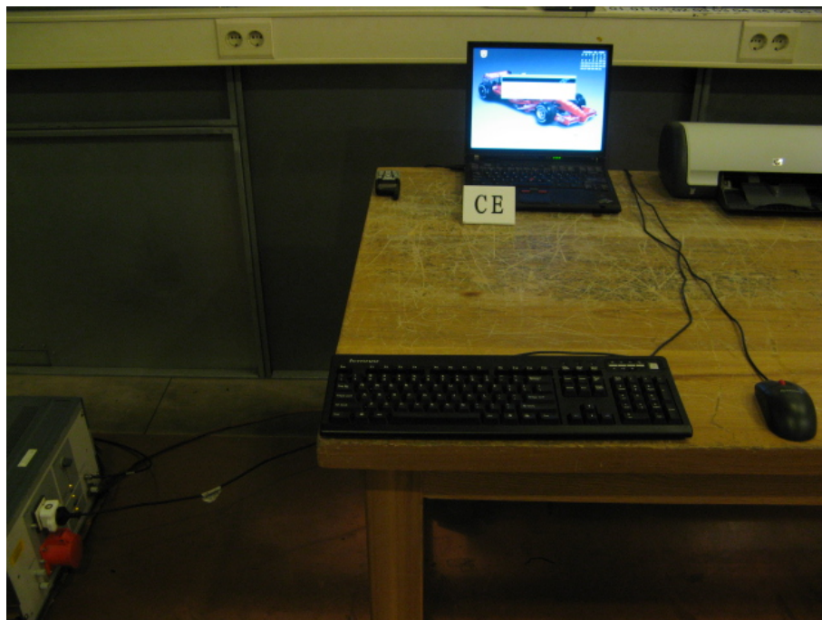
Pic C-2 Conducted Emission (USB Mode)
