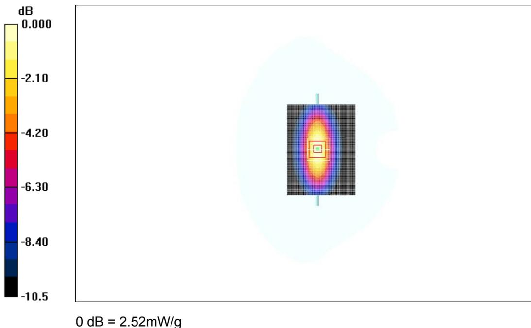
Figure 280 System Performance Check 835MHz 250mW
