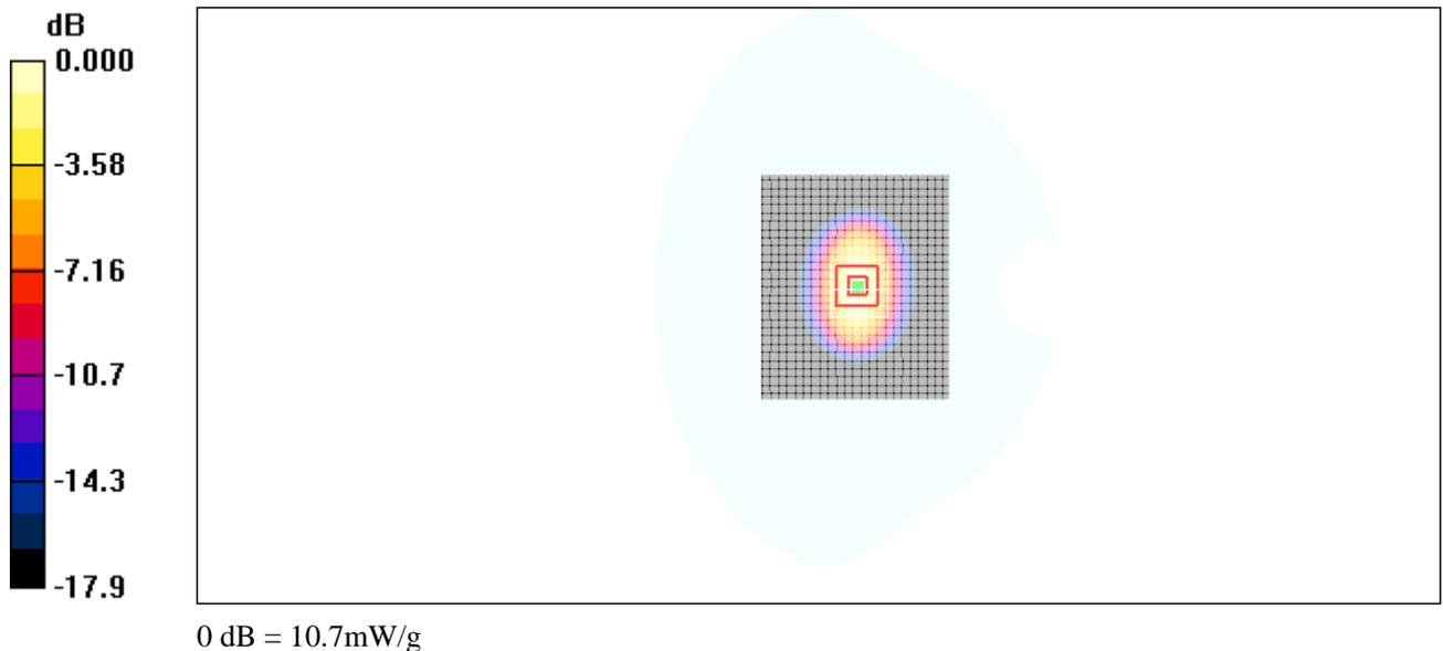
Figure 281 System Performance Check 1900MHz 250mW
