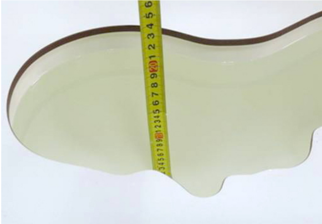
Picture 5: liquid depth in the head Phantom (1900 MHz)
