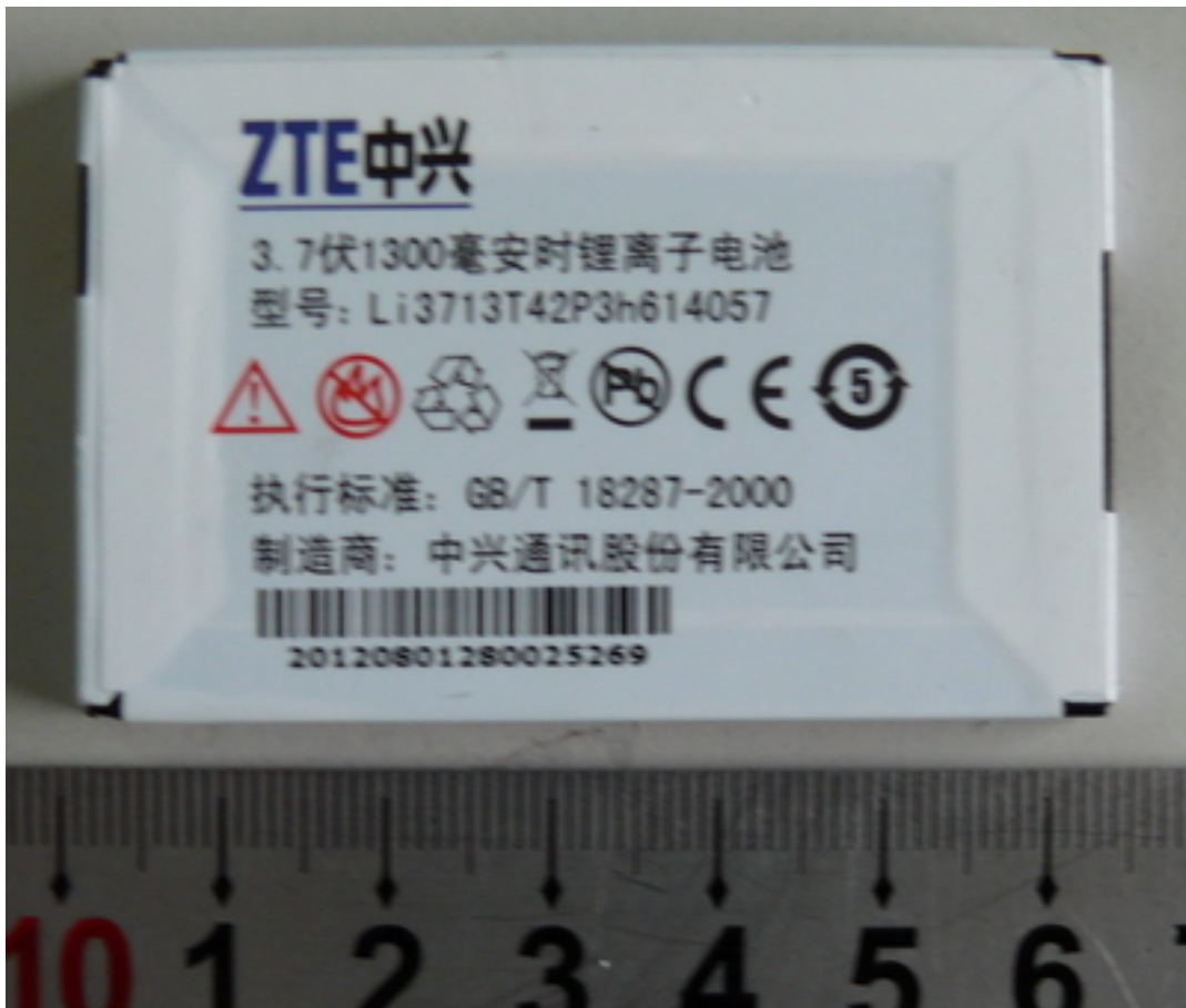
6-b: Battery - front view
