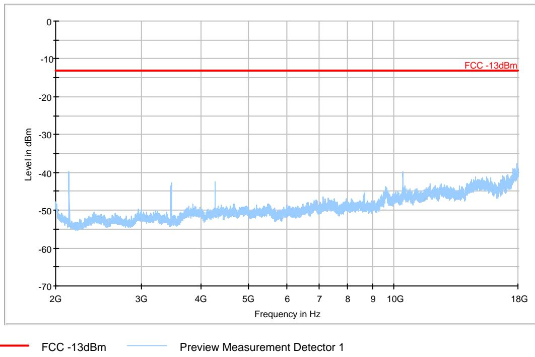
**A.2.3.14 RADIATED SPURIOUS EMISSIONS-Channel 875: 2GHz – 18GHz Set.1**
