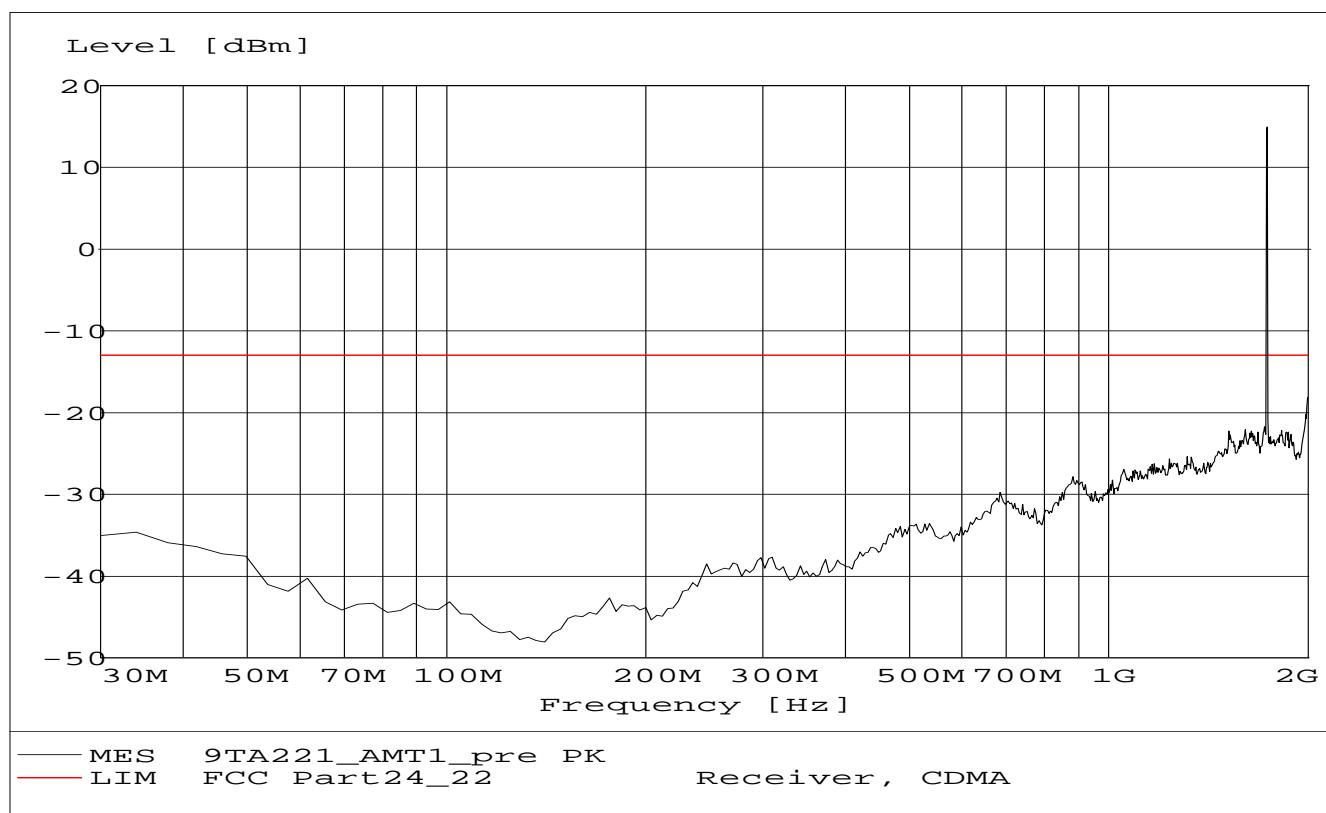
**A.2.3.11 RADIATED SPURIOUS EMISSIONS-Channel 875: 30MHz – 2GHz Set.1**
