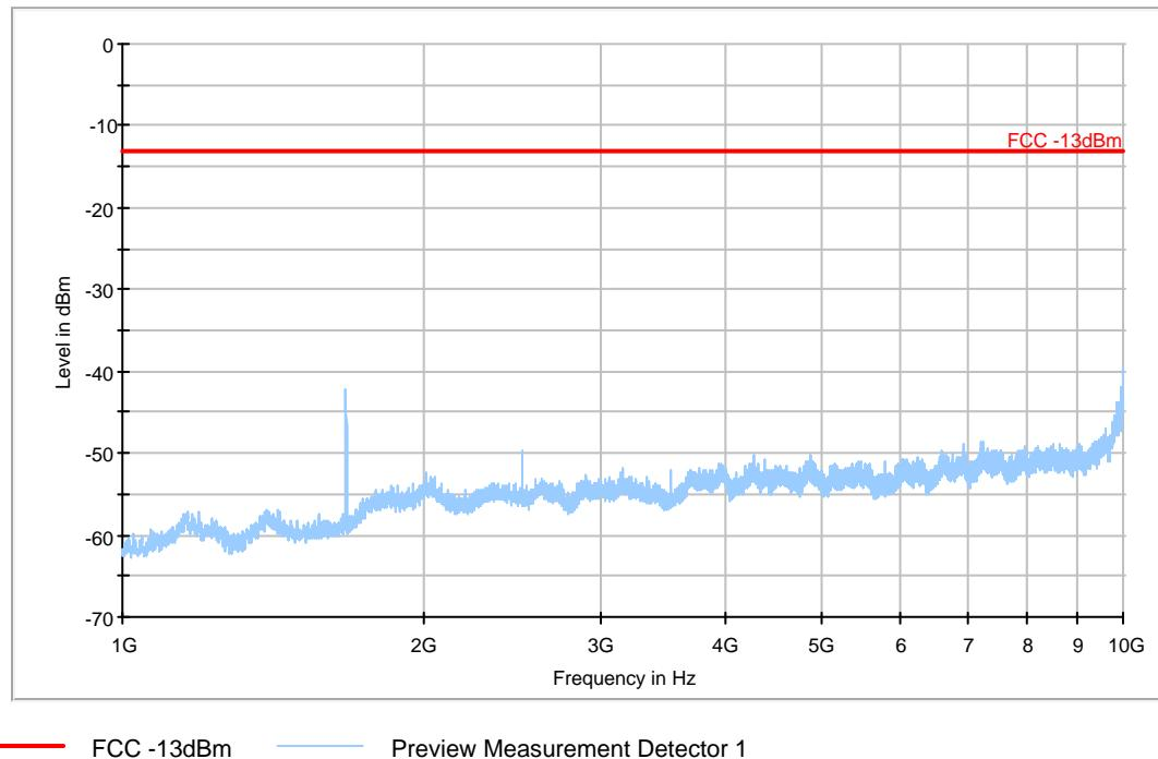
**A.2.3.6 RADIATED SPURIOUS EMISSIONS-Channel 777: 1GHz – 10GHz Set.1**
