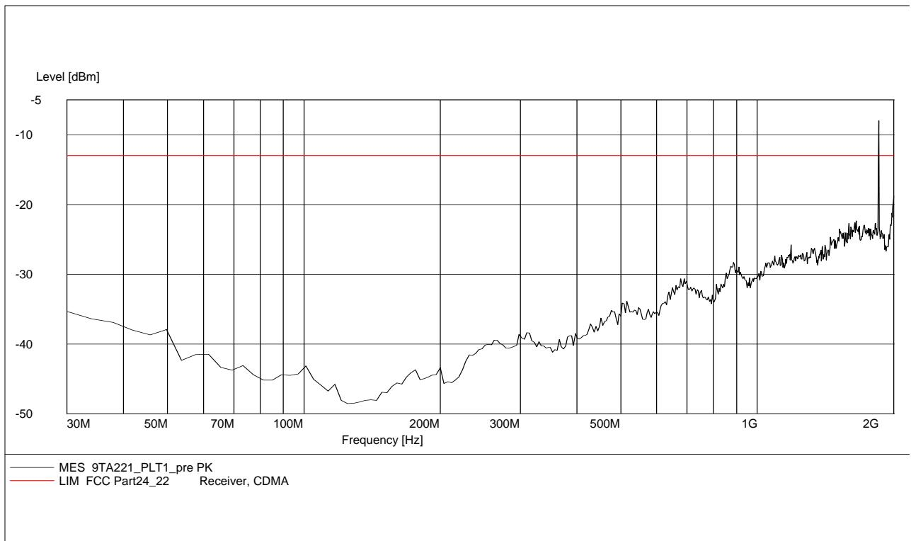
**A.2.3.20 RADIATED SPURIOUS EMISSIONS-Channel 600: 30MHz – 2GHz Set.1****NOTE: peak above the limit line is the Carrier frequency @ ch-600**
