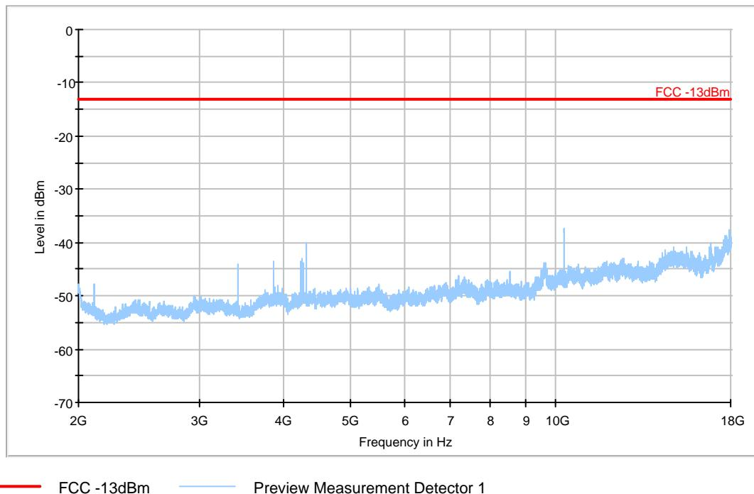
**A.2.3.13 RADIATED SPURIOUS EMISSIONS-Channel 450: 2GHz – 18GHz Set.1**
