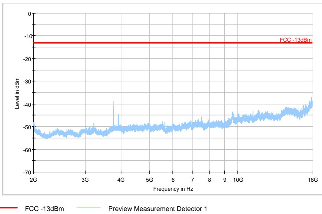
**A.2.3.24 RADIATED SPURIOUS EMISSIONS-Channel 1175: 2GHz – 18GHz Set.1**
