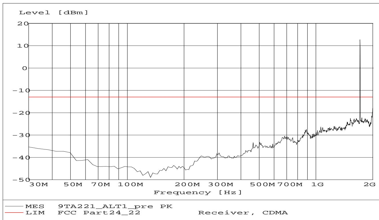
**A.2.3.10 RADIATED SPURIOUS EMISSIONS-Channel 450: 30MHz – 2GHz Set.1****NOTE: peak above the limit line is the Carrier frequency @ ch-450**
