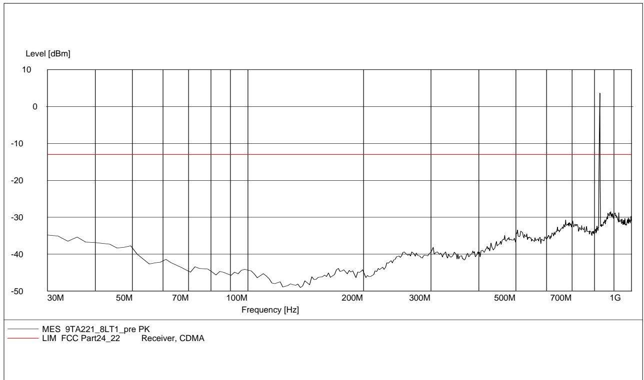
**A.2.3.2 RADIATED SPURIOUS EMISSIONS-Channel 384: 30MHz – 1GHz Set.1****Radiated spurious emission limit :-13dBm.****NOTE: peak above the limit line is the Carrier frequency @ ch-384**
