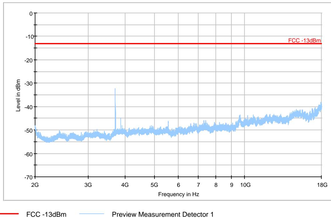
**A.2.3.23 RADIATED SPURIOUS EMISSIONS-Channel 600: 2GHz – 18GHz Set.1**
