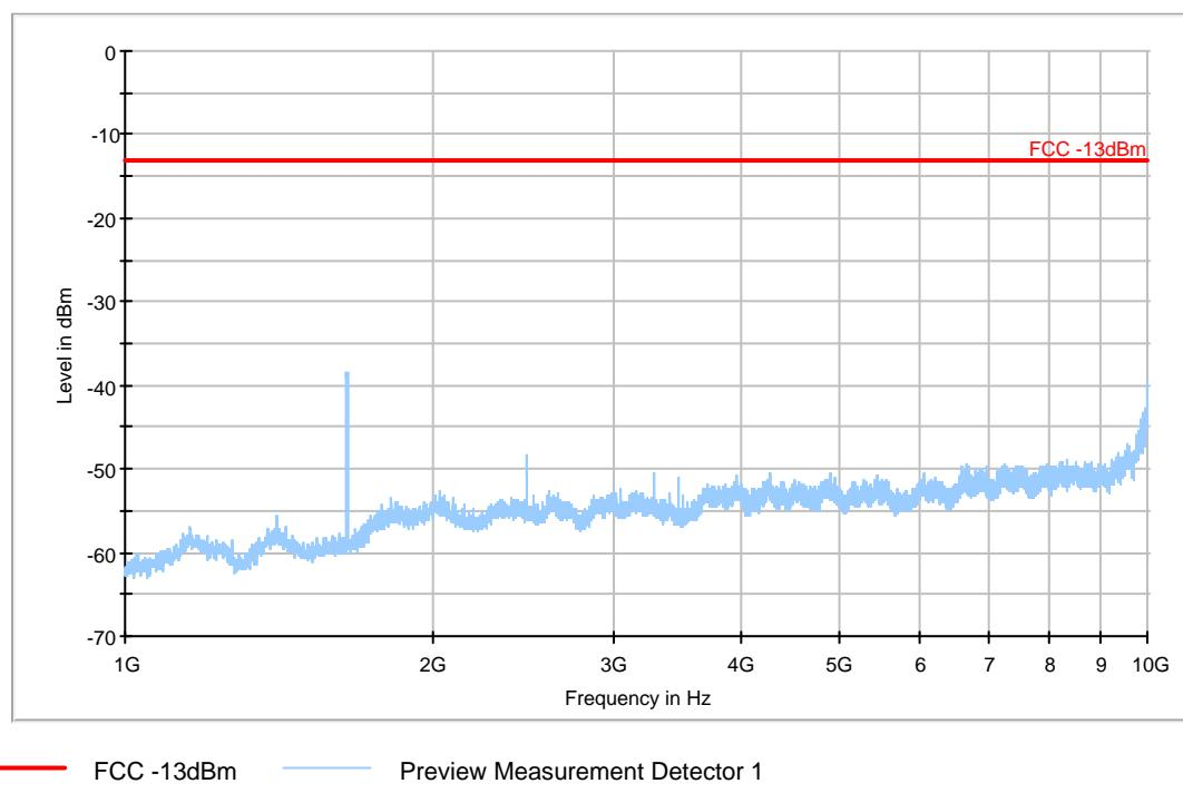
**A.2.3.5 RADIATED SPURIOUS EMISSIONS-Channel 384: 1GHz – 10GHz Set.1**
