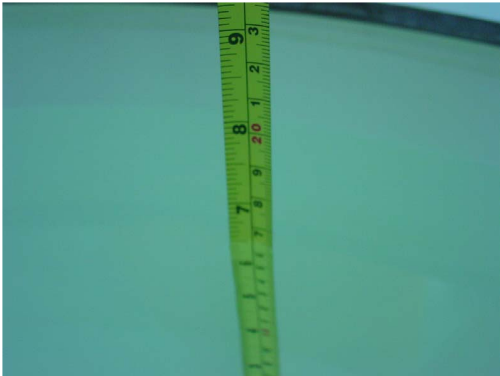
Picture B4 Liquid depth in the Flat Phantom (1800MHz)
