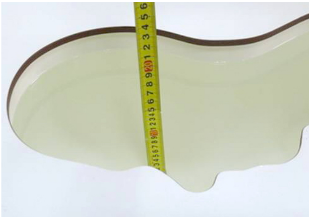
Picture 4: liquid depth in the head Phantom (1900 MHz, 15.2cm depth)
