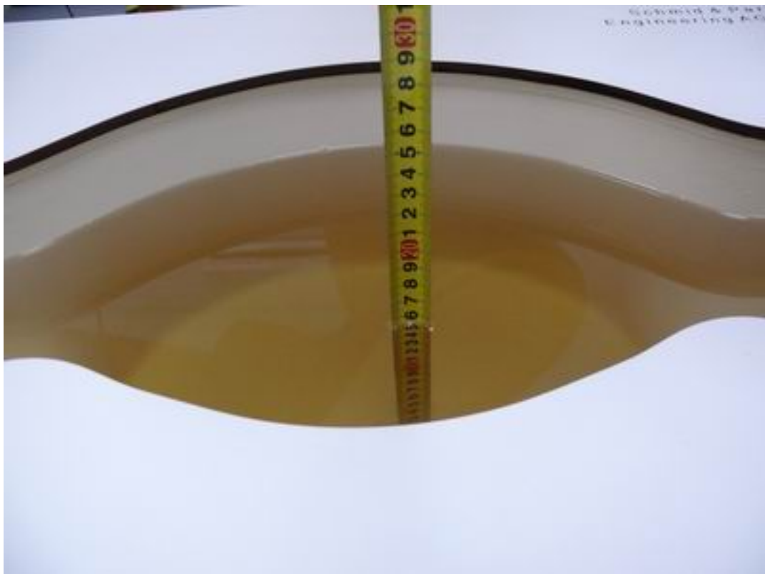
Picture 3: Liquid depth in the flat Phantom (835MHz, 15.3cm depth)
