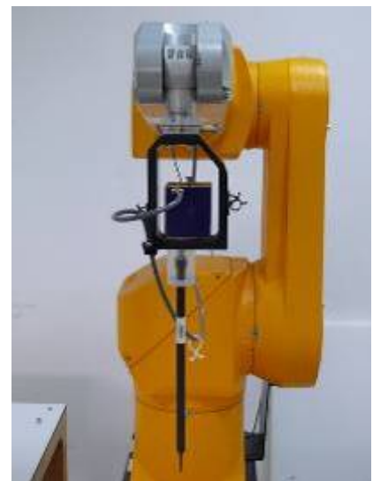
Figure 3. EX3DV4 E-field probe
