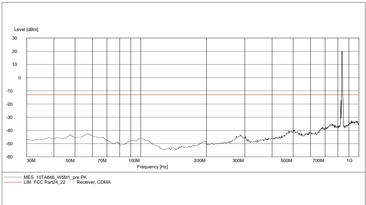
**A.2.3.13 RADIATED SPURIOUS EMISSIONS-Channel 4233: 30MHz – 1GHz****Radiated spurious emission limit :-13dBm.****NOTE: peak above the limit line is the Carrier frequency @ ch-4233**
