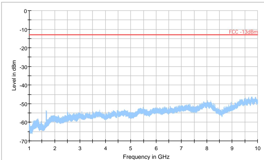
**A.2.3.16 RADIATED SPURIOUS EMISSIONS-Channel 4233: 1GHz – 10GHz**
