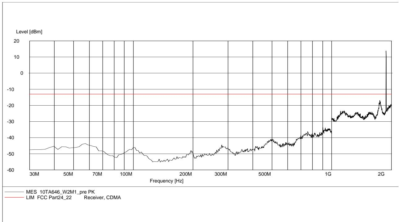
**A.2.3.3 RADIATED SPURIOUS EMISSIONS-Channel 9538: 30MHz – 2GHz****Radiated spurious emission limit :-13dBm.****NOTE: peak above the limit line is the Carrier frequency @ ch-9538**
