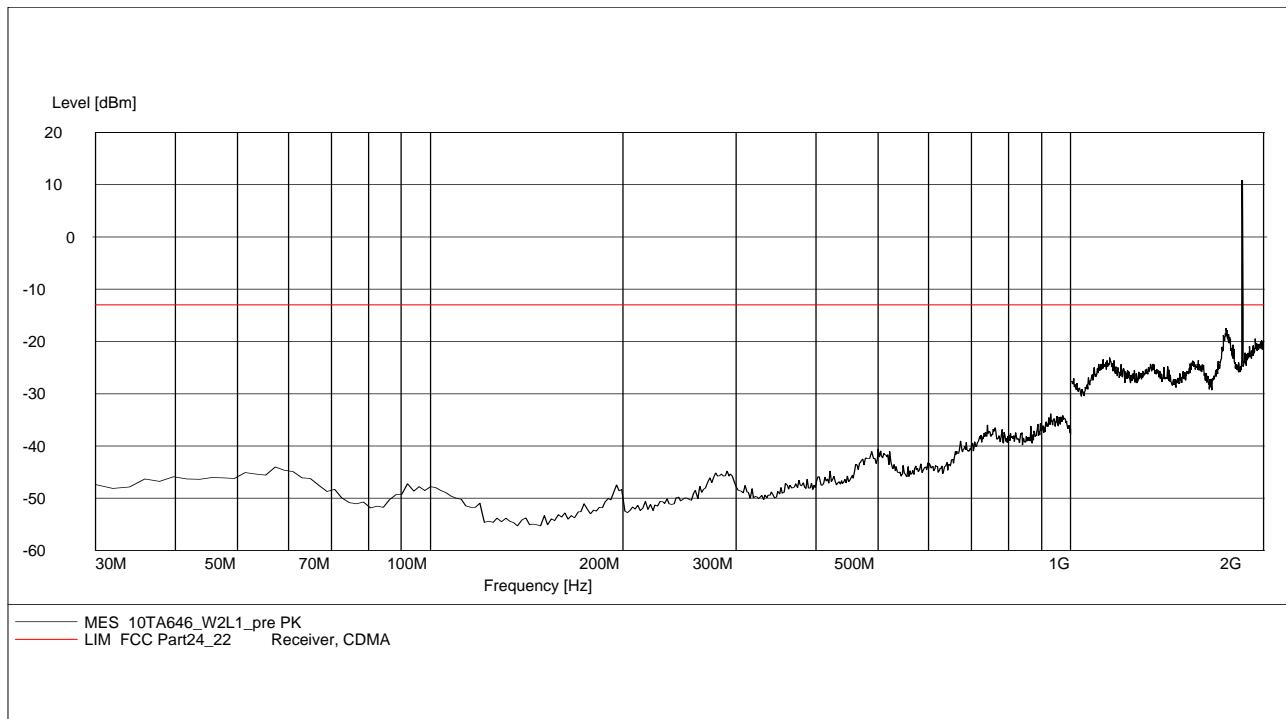
**A.2.3.2 RADIATED SPURIOUS EMISSIONS-Channel 9400: 30MHz – 2GHz****Radiated spurious emission limit :-13dBm.****NOTE: peak above the limit line is the Carrier frequency @ ch-9400**
