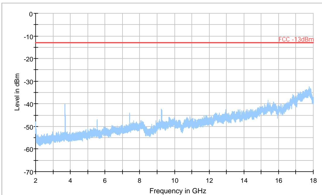
**A.2.3.5 RADIATED SPURIOUS EMISSIONS-Channel 9400: 2GHz – 18GHz****Radiated spurious emission limit :-13dBm.**
