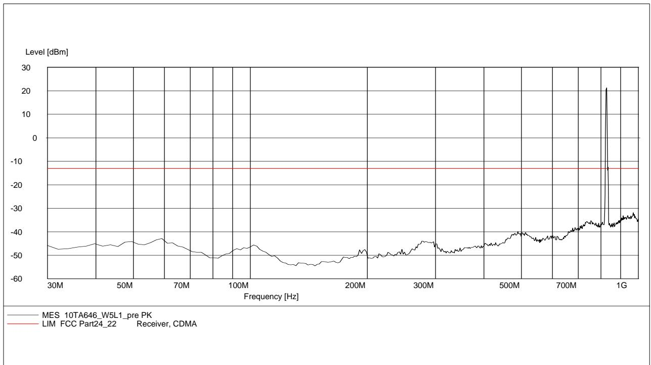
**A.2.3.12 RADIATED SPURIOUS EMISSIONS-Channel 4183: 30MHz – 1GHz****Radiated spurious emission limit :-13dBm.****NOTE: peak above the limit line is the Carrier frequency @ ch-4183**
