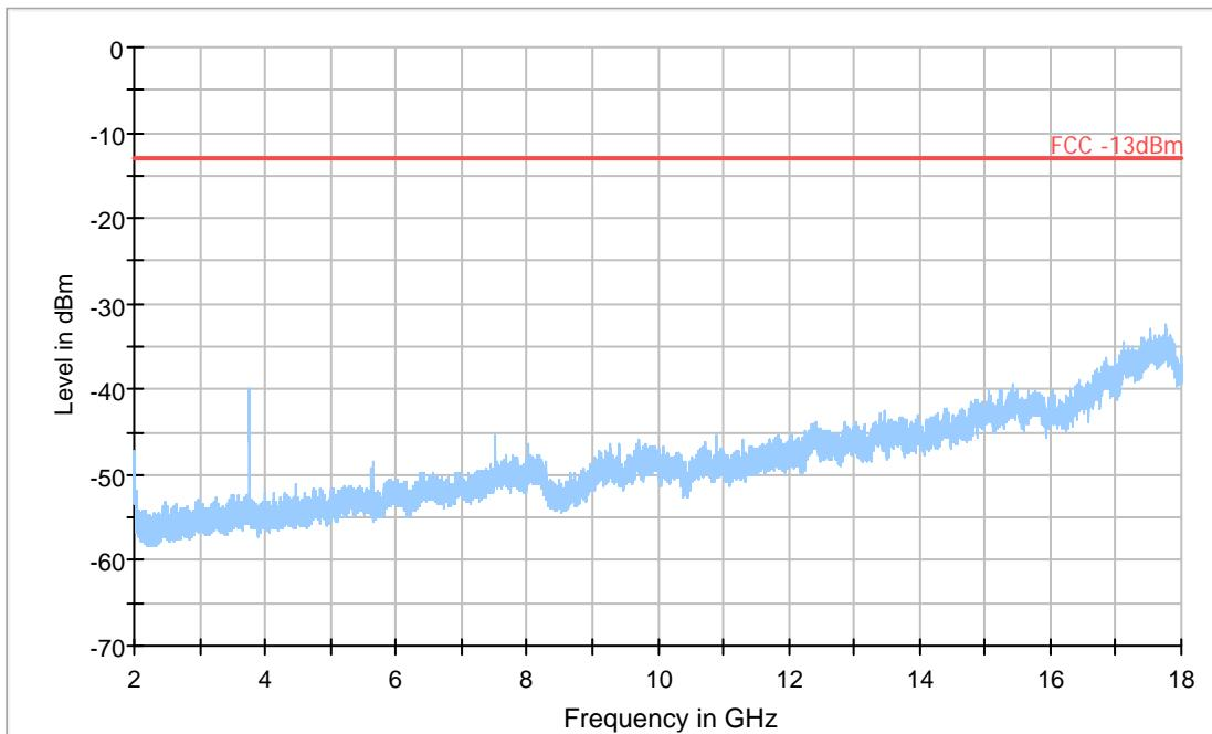
**A.2.3.6 RADIATED SPURIOUS EMISSIONS-Channel 9538: 2GHz – 18GHz****Radiated spurious emission limit :-13dBm.**
