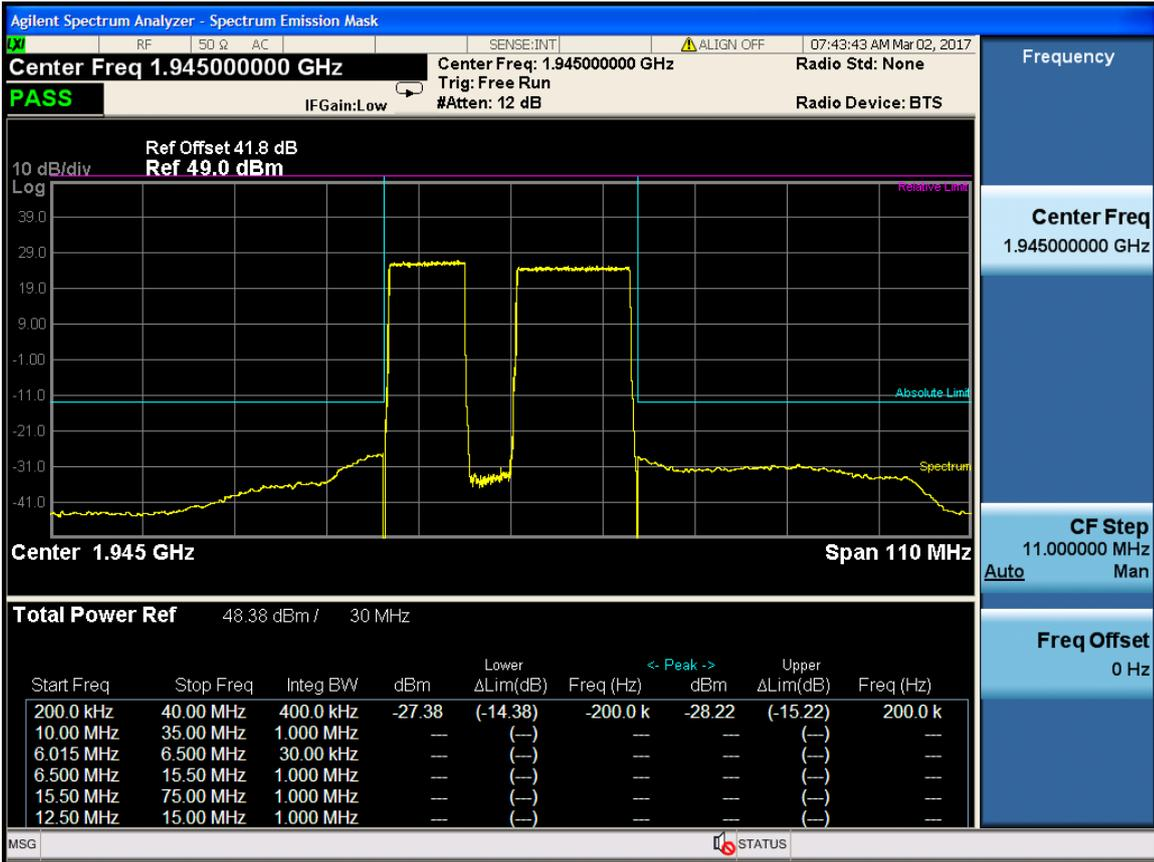
RF 30M(LTE 10M+LTE 15M) -Port 4-1960MHz
