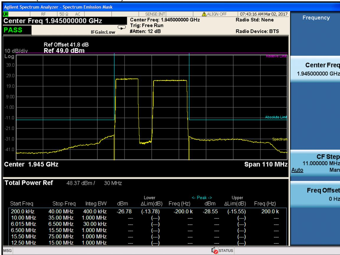
RF 30M(LTE 10M+LTE 15M) -Port 1-1960MHz
