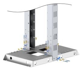
2. Fix the top beam to the posts with four M5 × 16 screws, see Figure 11-2.
