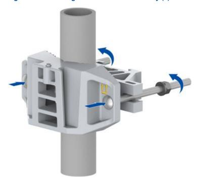
Figure 4-18 Installing the Pole Mount Assembly (2)
