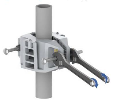
Figure 4-24 Installing the Pole Component (2)
