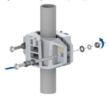
3. Tighten the nuts on both sides of the pole component with an adjustable wrench with a torque of 40 N m to fix the pole component on the pole, see Figure 4-24.
