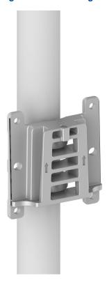
3. Mount the ZXSDR R8854 to the fixing clip on the pole along the rail of the fixing clip, see Figure 4-30.
