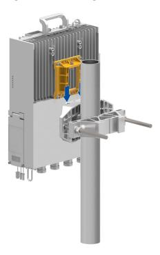
6. Tighten the captive screw on the RRU support with an M6 inner-hexagon wrench to fix the ZXSDR R8854, see Figure 4-21.
