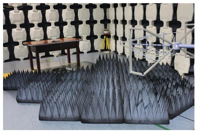
Fig.2 Radiated emission test (above 1 GHz)
