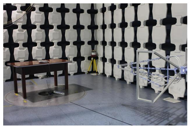
Fig.1 Radiated emission test (below 1 GHz)
