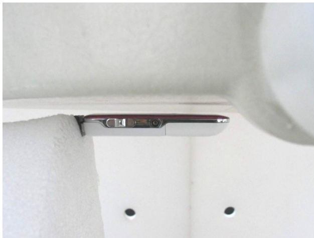
USB Cable Plug-in for USB Configuration 2 (Horizontal Down with Phantom 0.5 cm Gap)
