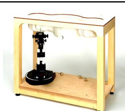
Fig 5.7 Photo of SAM Phantom
