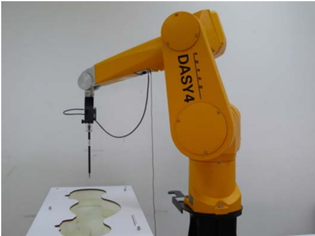
Picture 2: Specific Absorption Rate Test Layout
