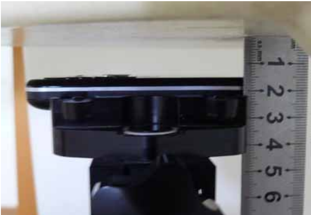
Picture 12: Body, display towards phantom, the distance from handset to the bottom of the Phantom is 15mm)
