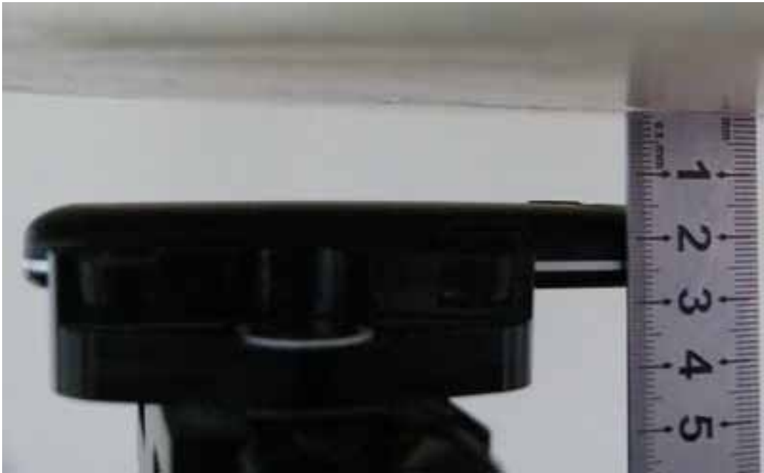
Picture 11: Body, The EUT display towards ground, the distance from handset to the bottom of the Phantom is 15mm)
