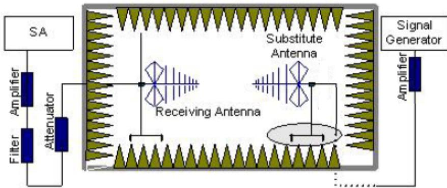
**For 850MHz working frequency test**
