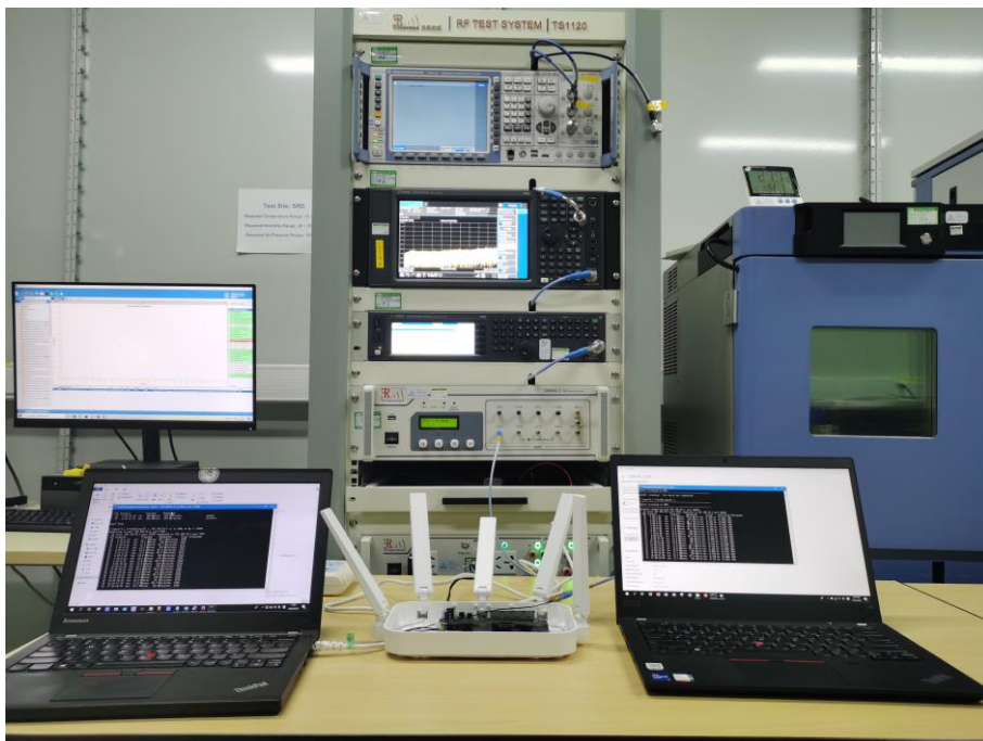
Photograph 4: Set-up photo for DFS test
