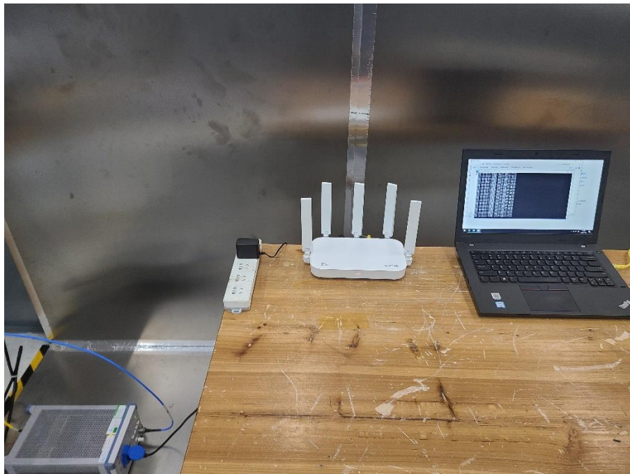
Photograph 4: Set-up photo for Conducted Emission
