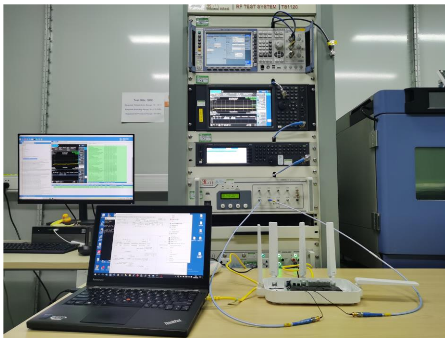
Photograph 3: Set-up photo for RF Conducted Singnal test
