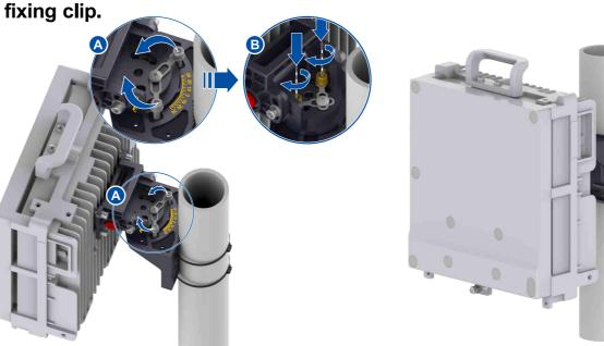
Installing the ZXSDR BS8922 on the Wall
