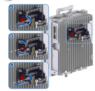
C Secure the vertical fastening screws.
