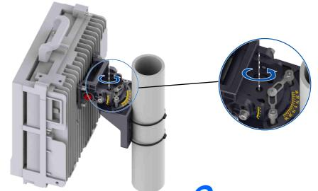
**b** Secure the two screws of the installation bracket on the fixing clip
