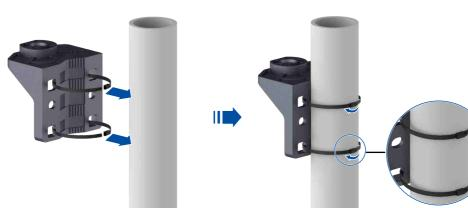
Mount the ZXSDR BS8922, on which the installation bracket is installed, on the fixing clip.
