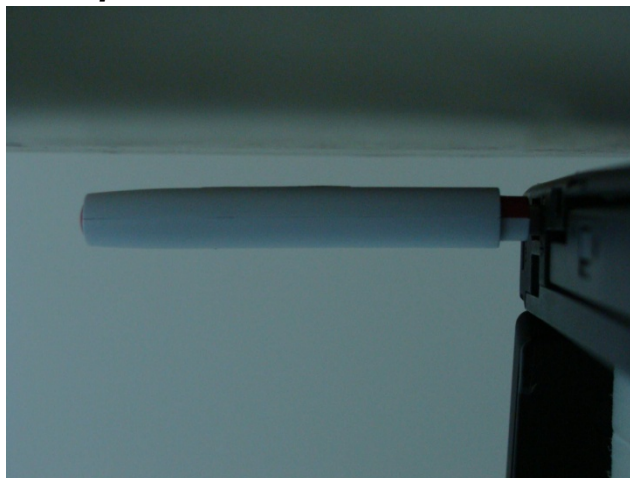
Direct Laptop Plug-in for USB Configuration 1 (Horizontal Down with Phantom 0.5 cm Gap)
