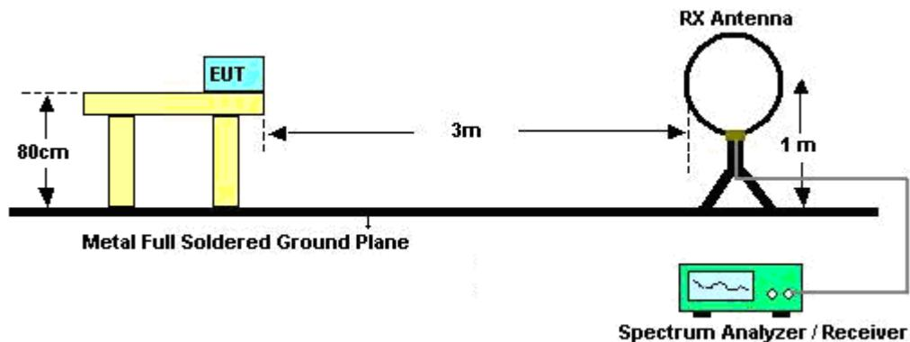
For radiated emissions from 30MHz to 1GHz
