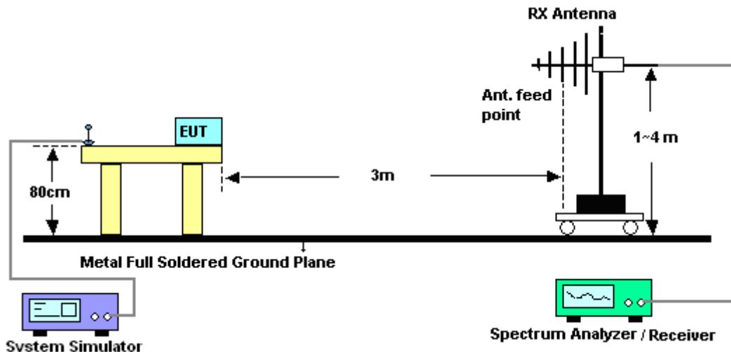
**For radiated emissions above 1GHz**
