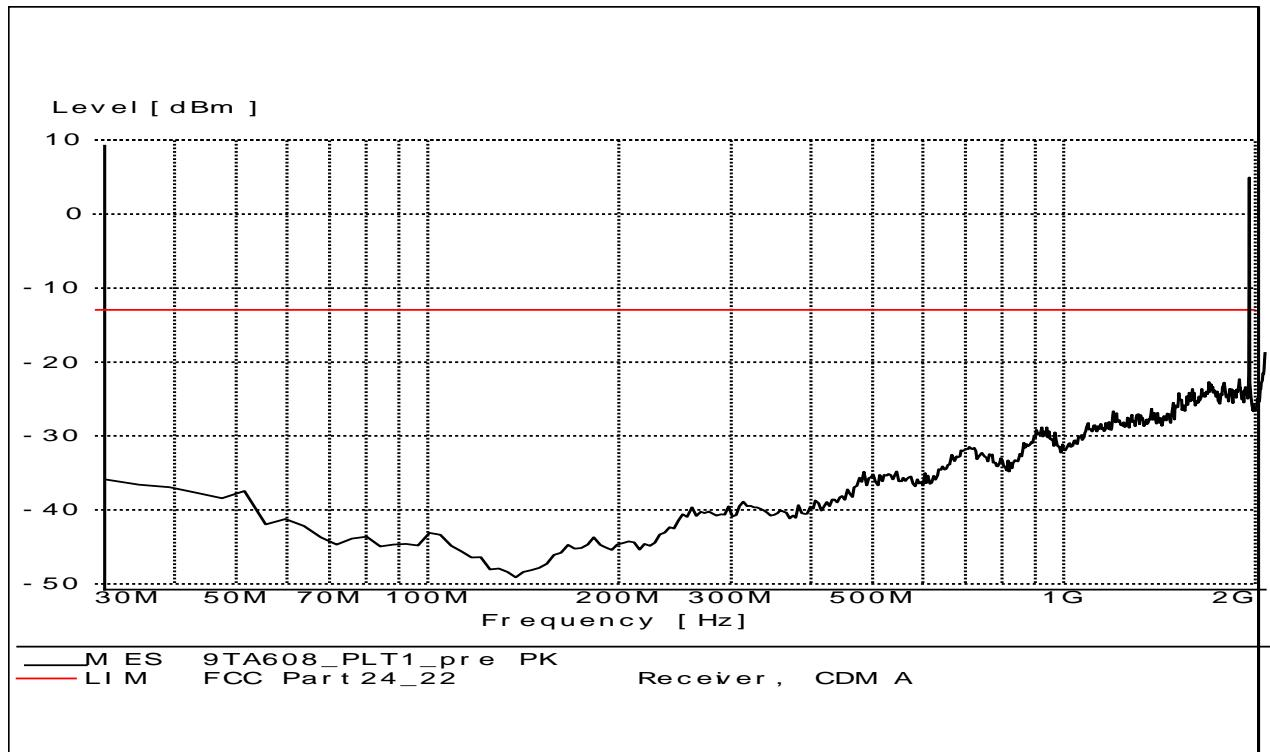
**A.2.3.10 RADIATED SPURIOUS EMISSIONS-Channel 661: 30MHz – 2GHz****Radiated spurious emission limit :-13dBm.****NOTE: peak above the limit line is the Carrier frequency @ ch-661**
