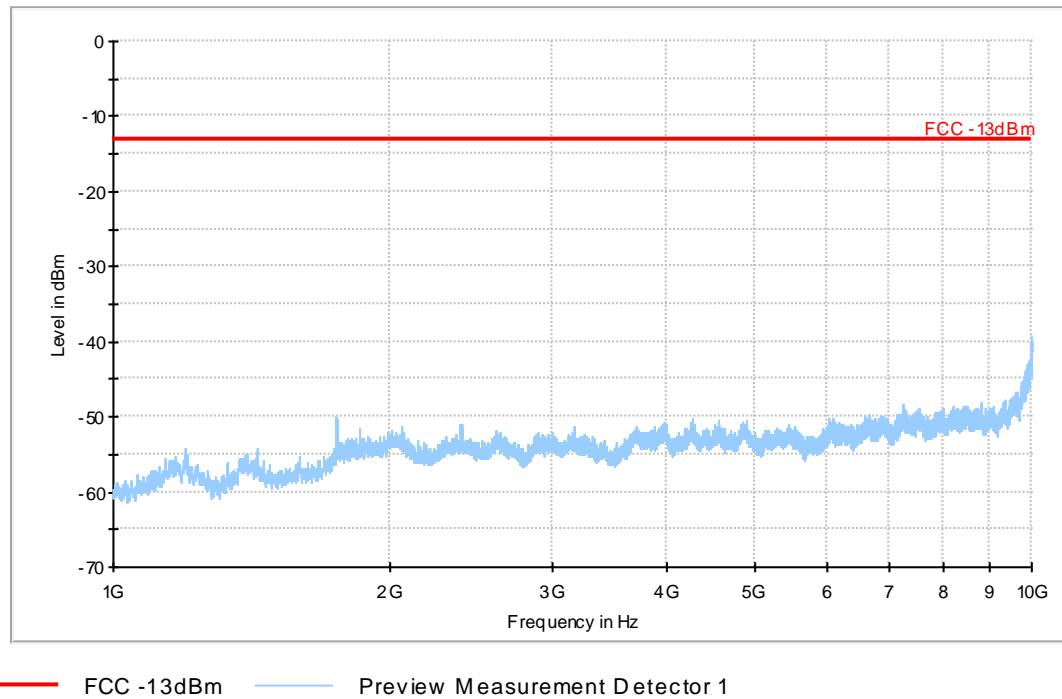
**A.2.3.6 RADIATED SPURIOUS EMISSIONS-Channel 251: 1GHz – 10GHz**
