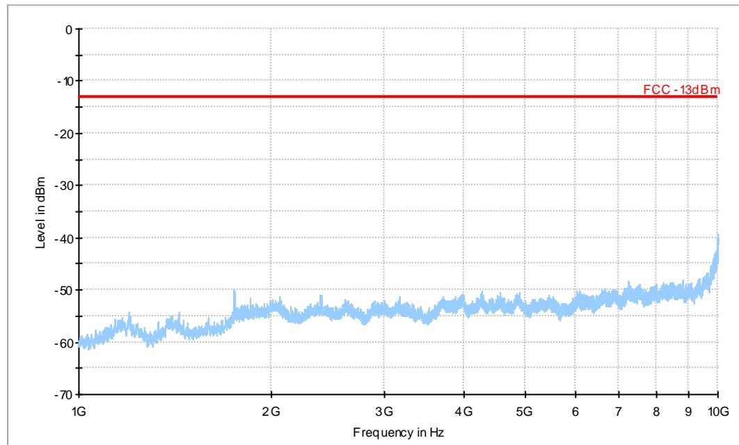
**A.2.3.5 RADIATED SPURIOUS EMISSIONS-Channel 190: 1GHz – 10GHz**
