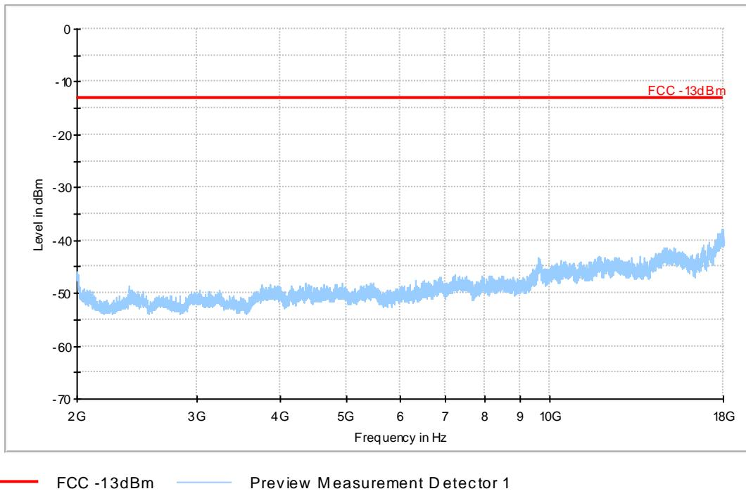
**A.2.3.14 RADIATED SPURIOUS EMISSIONS-Channel 810: 2GHz – 18GHz**
