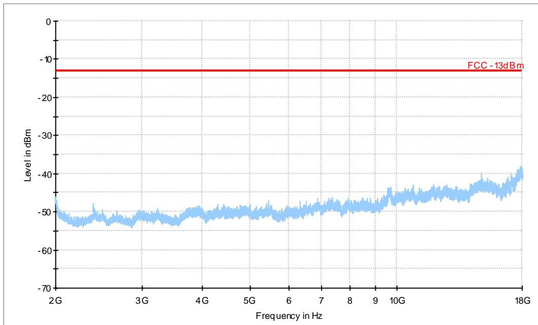
**A.2.3.13 RADIATED SPURIOUS EMISSIONS-Channel 661: 2GHz – 18GHz**
