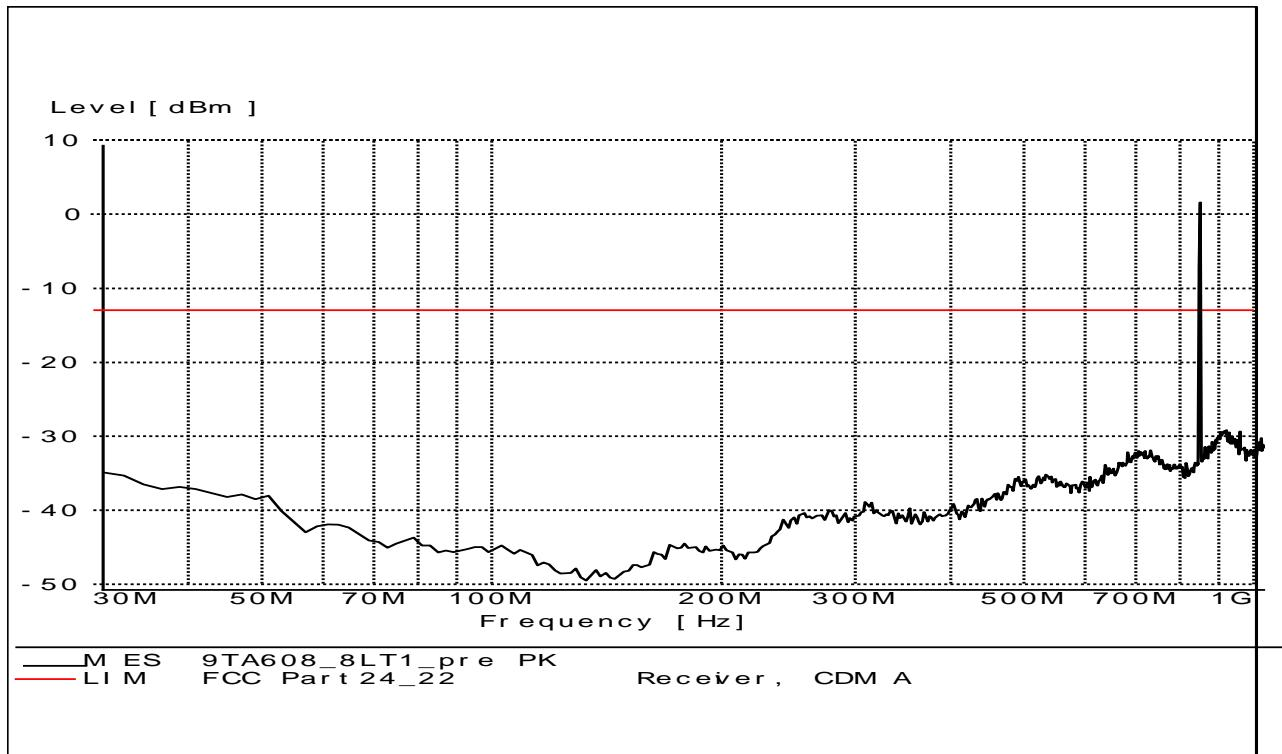
**A.2.3.2 RADIATED SPURIOUS EMISSIONS-Channel 190: 30MHz – 1GHz****Radiated spurious emission limit :-13dBm.****NOTE: peak above the limit line is the Carrier frequency @ ch-190**
