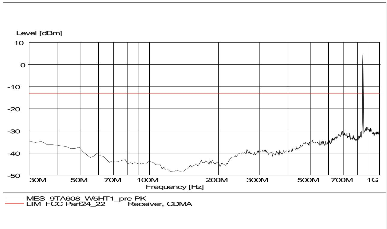
**A.2.3.14 RADIATED SPURIOUS EMISSIONS-Channel 4132: 1GHz – 10GHz****Radiated spurious emission limit :-13dBm.**
