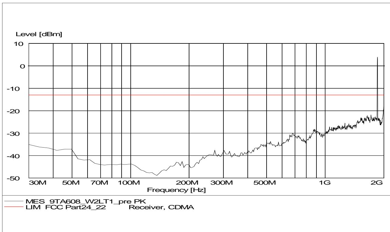
**A.2.3.2 RADIATED SPURIOUS EMISSIONS-Channel 9400: 30MHz – 2GHz**
