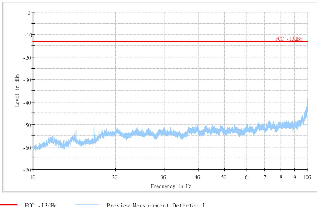
**A.2.3.16 RADIATED SPURIOUS EMISSIONS-Channel 4233: 1GHz – 10GHz**
