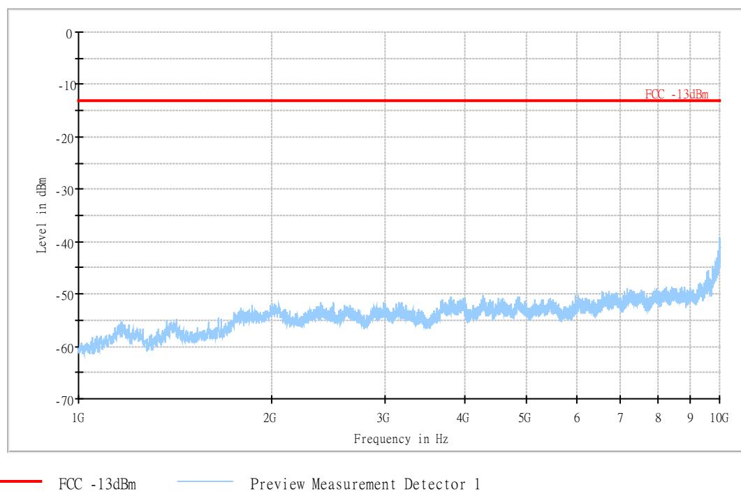
**A.2.3.15 RADIATED SPURIOUS EMISSIONS-Channel 4183: 1GHz – 10GHz**
