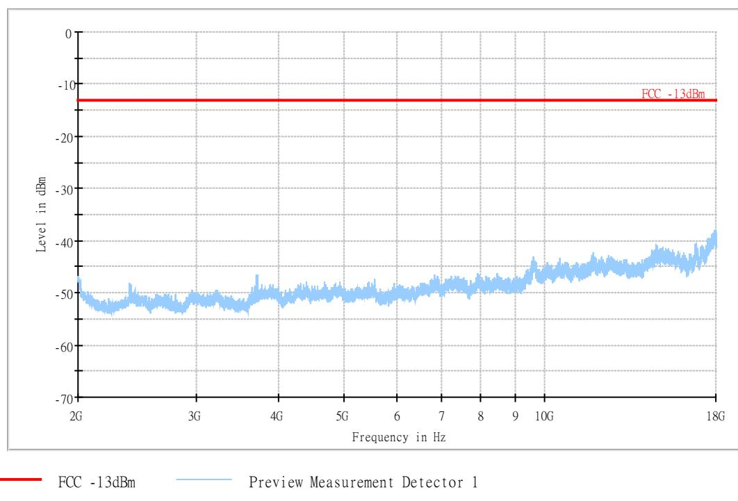
**A.2.3.5 RADIATED SPURIOUS EMISSIONS-Channel 9400: 2GHz – 18GHz**
