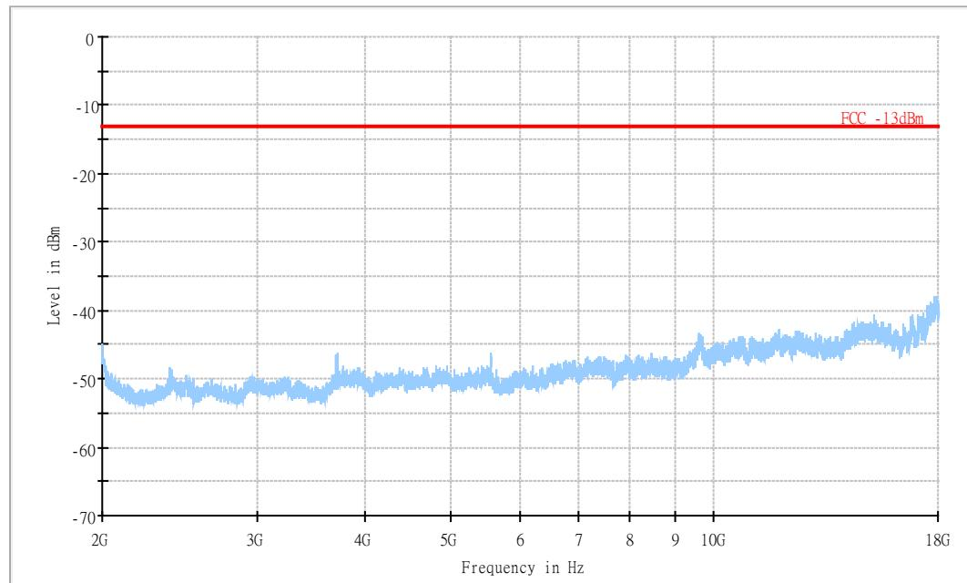
**A.2.3.6 RADIATED SPURIOUS EMISSIONS-Channel 9538: 2GHz – 18GHz**
