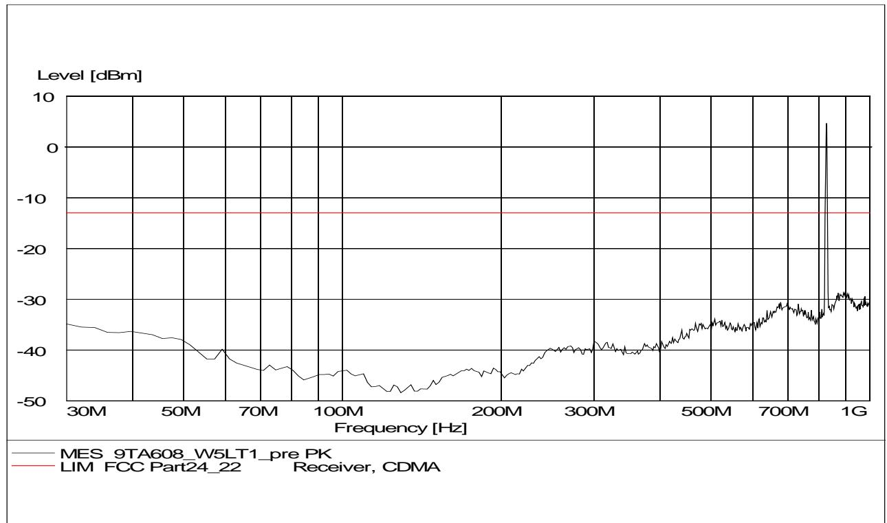
**A.2.3.12 RADIATED SPURIOUS EMISSIONS-Channel 4183: 30MHz – 1GHz****Radiated spurious emission limit :-13dBm.****NOTE: peak above the limit line is the Carrier frequency @ ch-4183**
