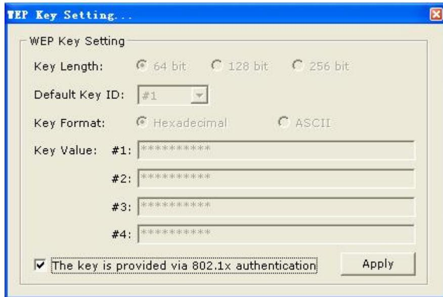
**The key is provided via IEEE 802.1X authentication:** Place a check in this box if IEEE 802.1X authentication is used. By selecting this option, the WEP key settings will be disabled.
