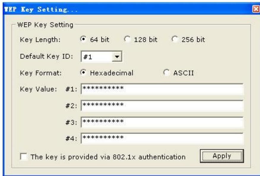
**Key Length:** Select an encryption key length: **64, 128 or 256 bit**. The setting must be the same as the Access Point.
