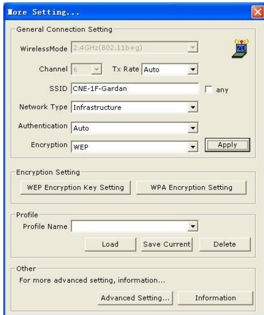
**SSID:** Enter the SSID of the network. The SSID is a unique name shared among all points in your wireless network. The SSID must be identical for all points in the network, and is case-sensitive. Place a check in the **any** box if you would like the device to connect to the first available Access Point with the strongest signal.
