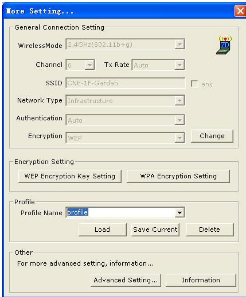
**Profile Name:** Displays the name of current profile. One device can have many profiles, but only one profile can be loaded at a time.
