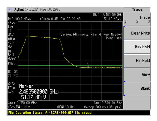
Detector mode: Peak Polarity: Horizontal
