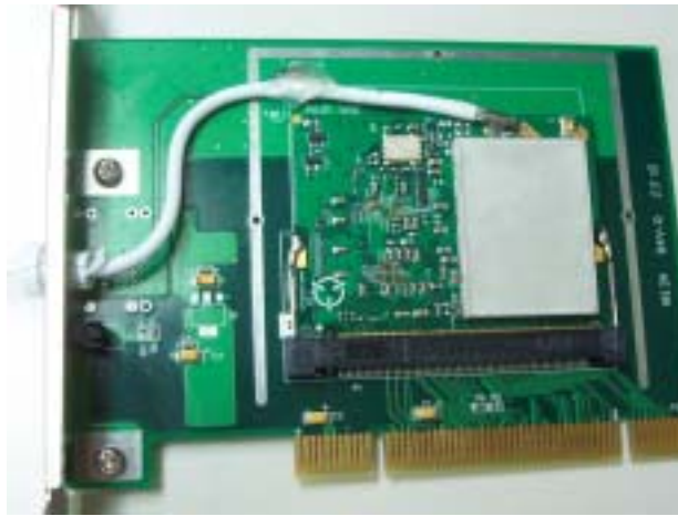
Fig. 1 PCI WLAN Card (with MiniPCI Module WLG500-3B and the integral antenna)
