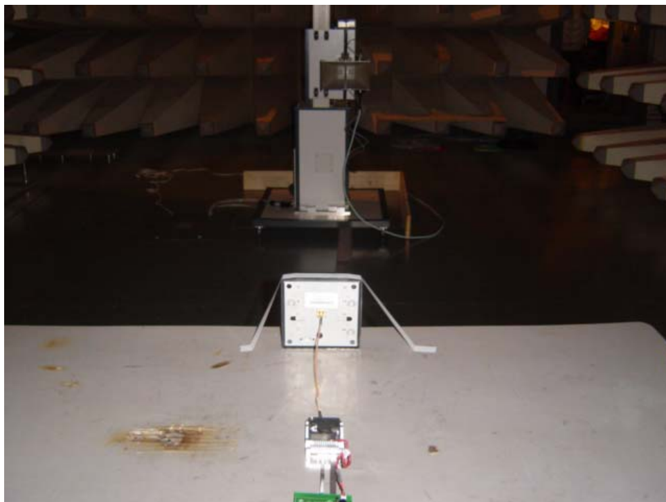
Test Setup of Radiated Emission Test
