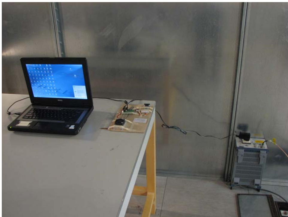
Test Setup of Conducted Emission Test
