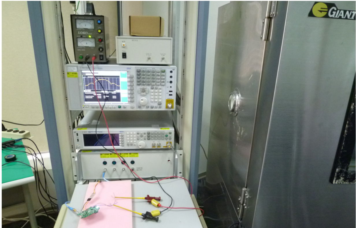
Photograph 4: Set-up for Conducted testing
