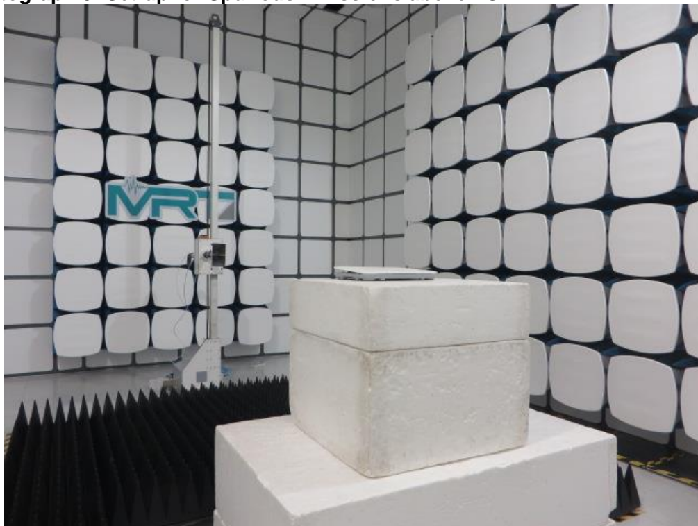
Photograph 3: Set-up for Spurious Emissions above 1GHz
