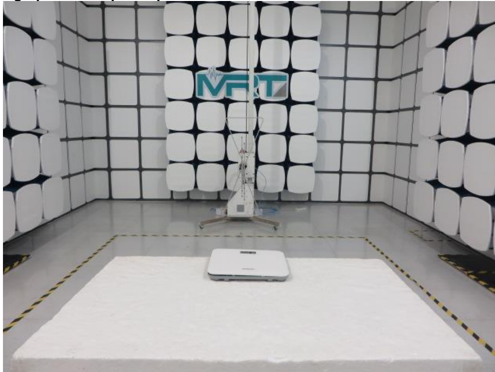
Photograph 2: Set-up for Spurious Emissions below 1GHz
