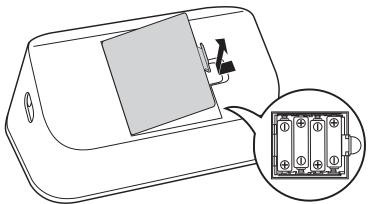
2. Insert 4 "AA" batteries as indicated in the battery compartment.
