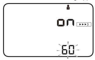
4. Press the or button to change the interval. It can be set 15, 30, 60, or 120 seconds.
