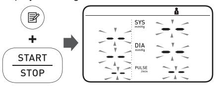
4. While holding the button down, press and hold the [START/STOP] button for more than 3 seconds.
