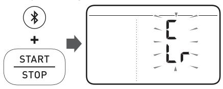
2. While holding the ③ button down, press and hold the [START/STOP] button for more than 3 seconds.
