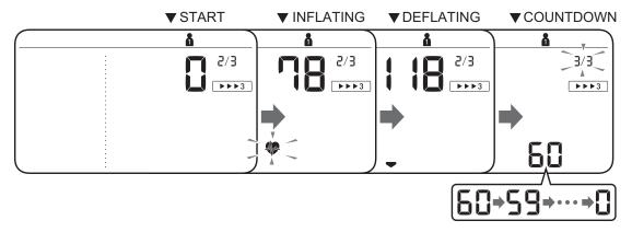
After the third measurement is complete, the average for the 3 measurements appears on the display.
