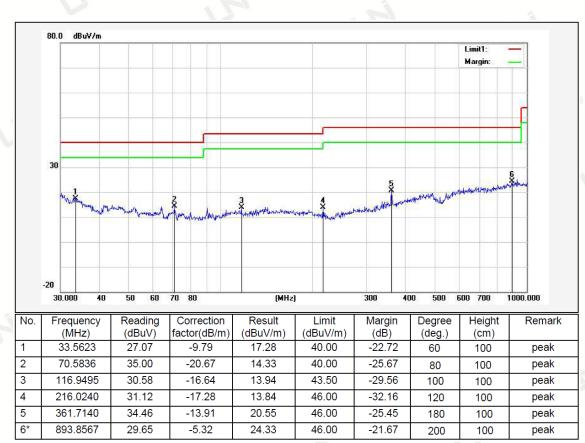
Remark: Absolute Level = Reading Level + Factor, Margin = Absolute Level – Limit Factor = Ant. Factor + Cable Loss – Pre-amplifier
