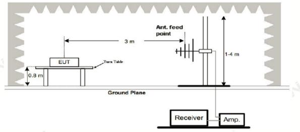
3. Radiated Emission Test-Up Frequency Above 1GHz
