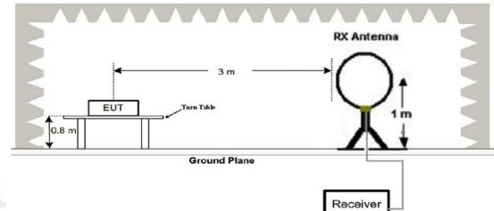
2. Radiated Emission Test-Up Frequency 30MHz~1GHz
