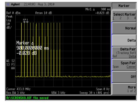
Alarm Transmitting Under Quickly Leak Silent Time =0.9-0.0285=0.8715s
