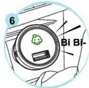
Display turn green, then " Bi " twice to enter the working mode
