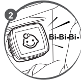
2 Display will "Bi" three times, the warning light will turn to red
