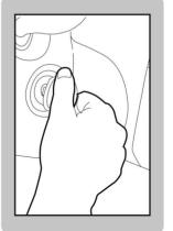
Turn the ignition key from OFF to ON for 5 times and keep in ON position at last time. The system will enter Bluetooth pairing mode.
