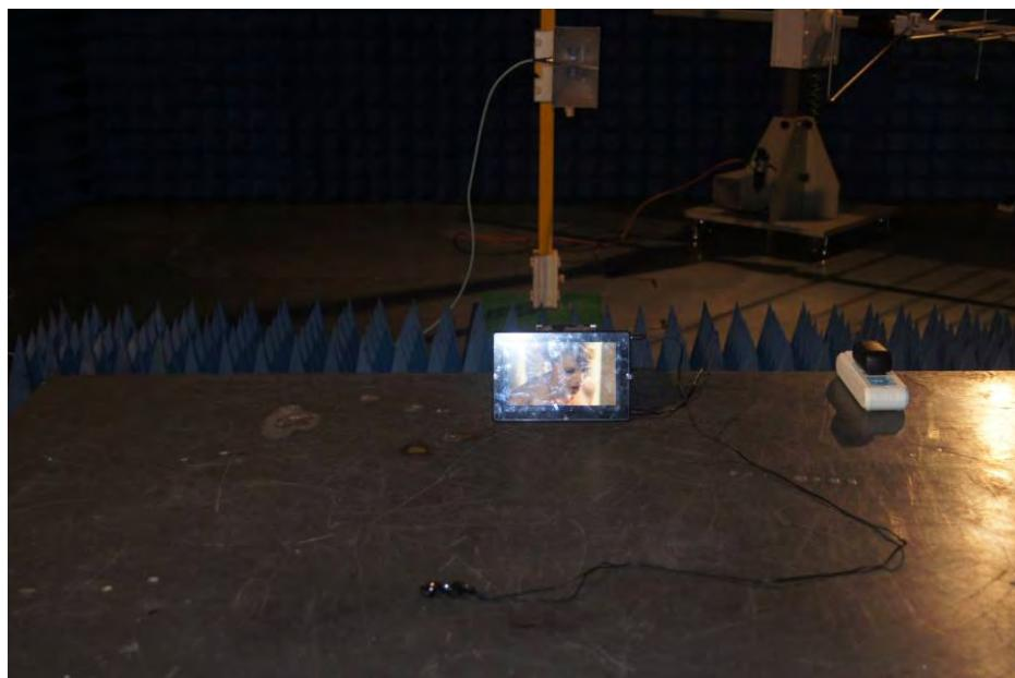
Radiated emission (up to 1G Transfer data mode):
