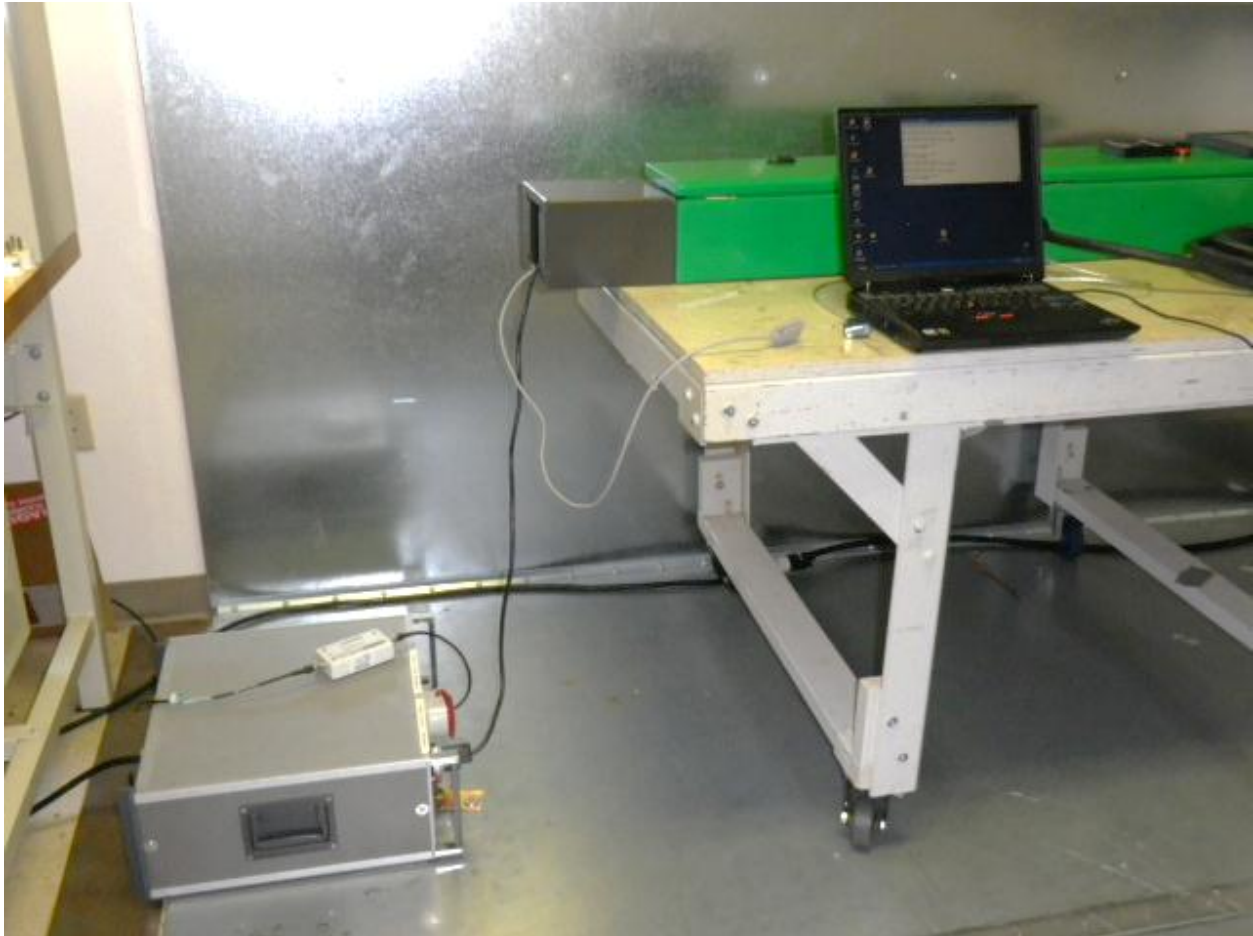
Figure 7: Conducted Emissions on AC Power Line. The Laptop is used to control the transmitter.
