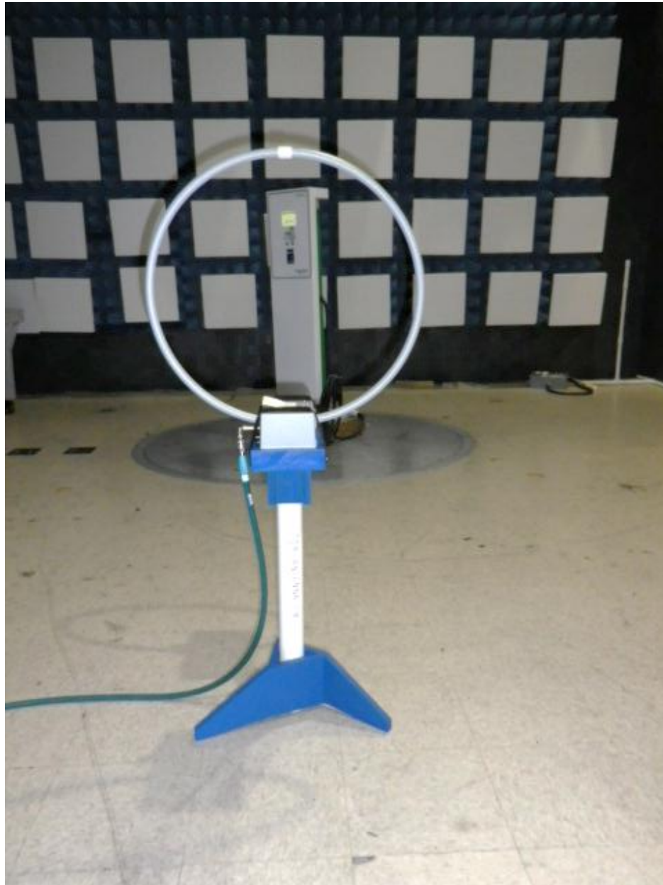
Figure 1: Typical Radiated Emissions – 10 kHz to 30 MHz for RFID transmitter. 3m in Chamber.
