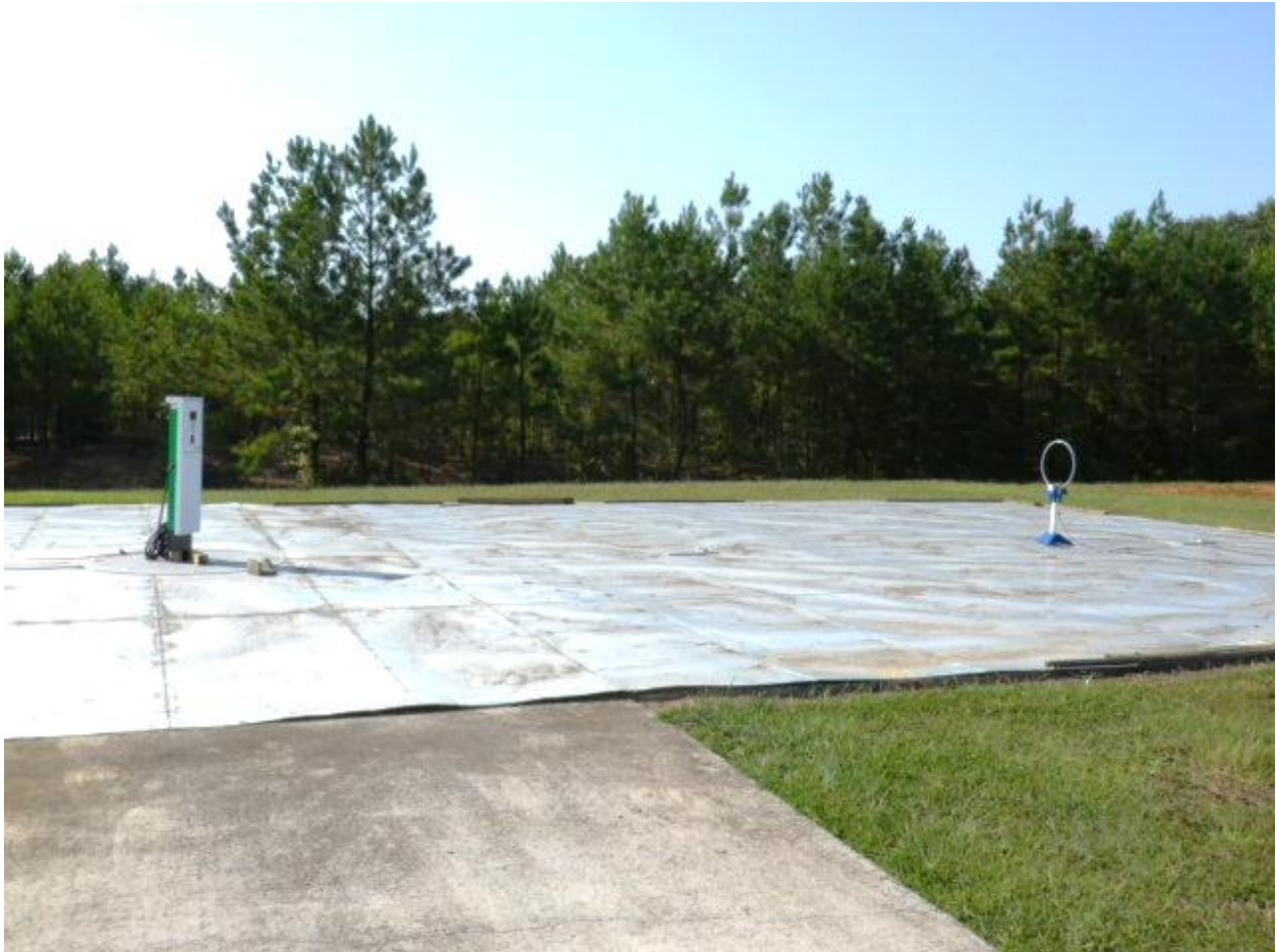
Figure 3: Verifying signal at 10m in the OATS.
