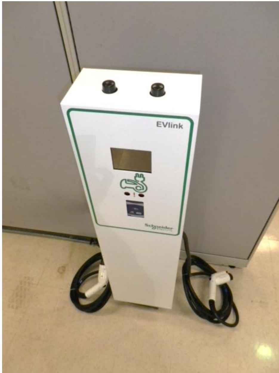
Figure 3: Top view of EUT showing external GSM and Zigbee antennas
