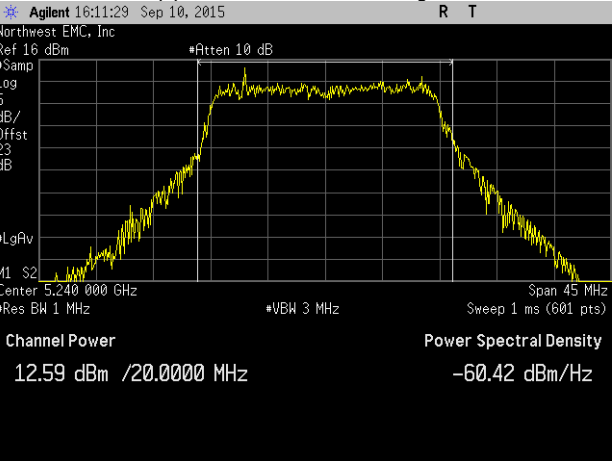
Chain B, 802.11(n) HT, MCS23, 20 MHz, High Channel 5240 MHz
