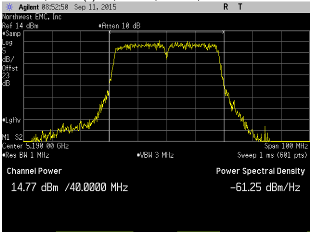
Chain A, 802.11(n) HT, MCS16, 40 MHz, Low Channel 5190 MHz
