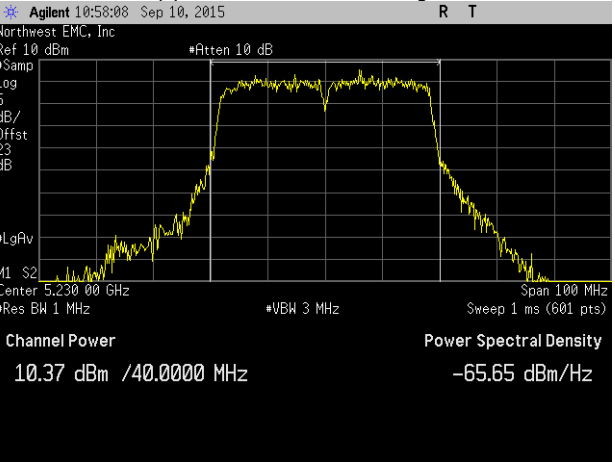
Chain A, 802.11(n) HT, MCS15, 40 MHz, High Channel 5230 MHz
