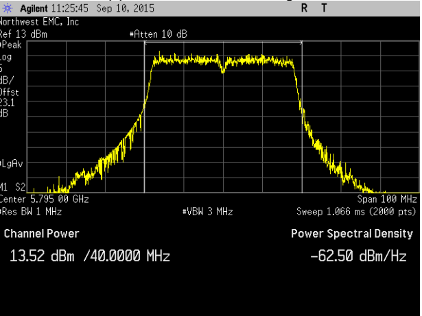
Chain A, 802.11(n) HT, MCS15, 40 MHz, High Channel 5795 MHz
