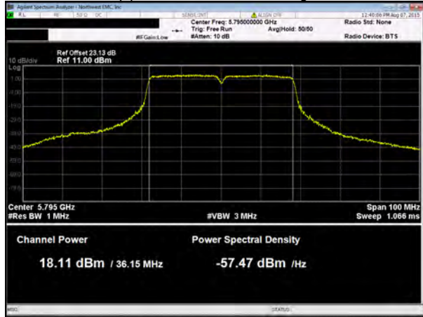
Chain C, 802.11(n) HT, MCS16, 40 MHz, High Channel 5795 MHz
