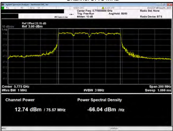
Chain A, 802.11(ac) VHT, MCS9 (256-QAM), 80 MHz, Low Channel 5775 MHz
