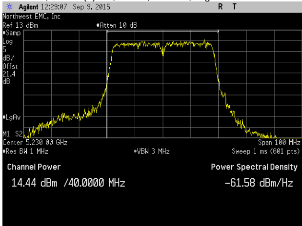
Chain C, 802.11(n) HT, MCS0, 40 MHz, High Channel 5230 MHz
