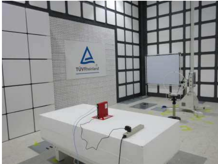
Photograph 5: Set-up for Spurious Emissions (Back View 3)
