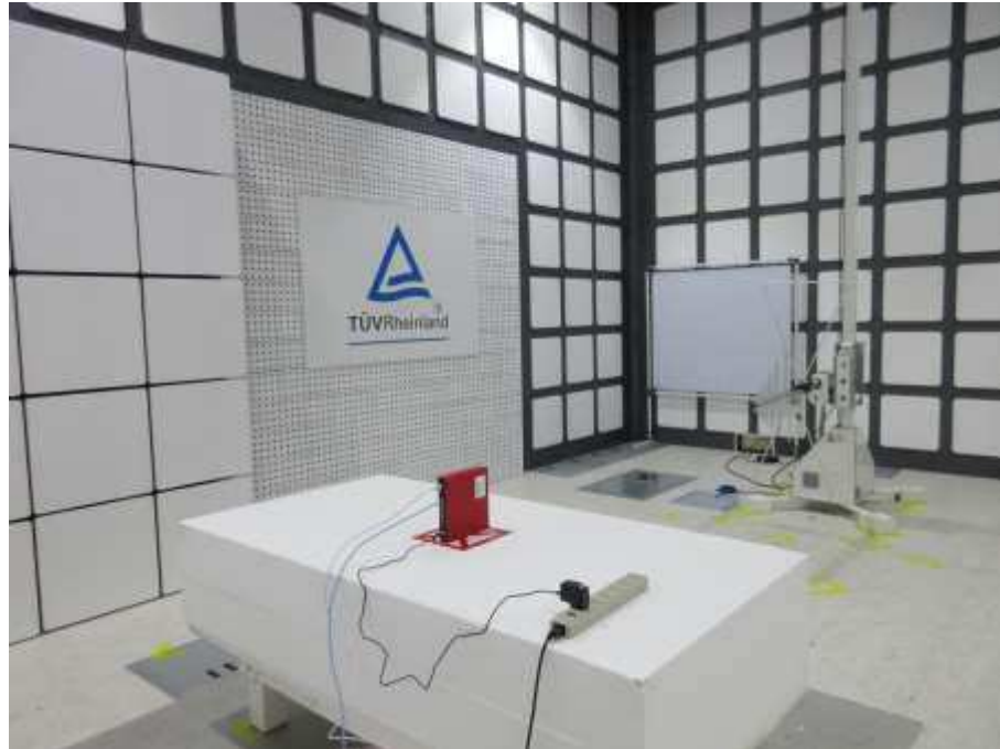
Photograph 4: Set-up for Spurious Emissions (Back View 2)
