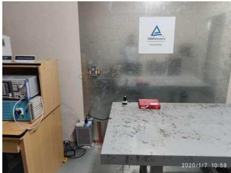
Photograph 6: Set-up for Mains Conducted testing (Front View)
