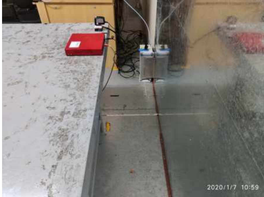
Photograph 7: Set-up for Mains Conducted testing (Back View)
