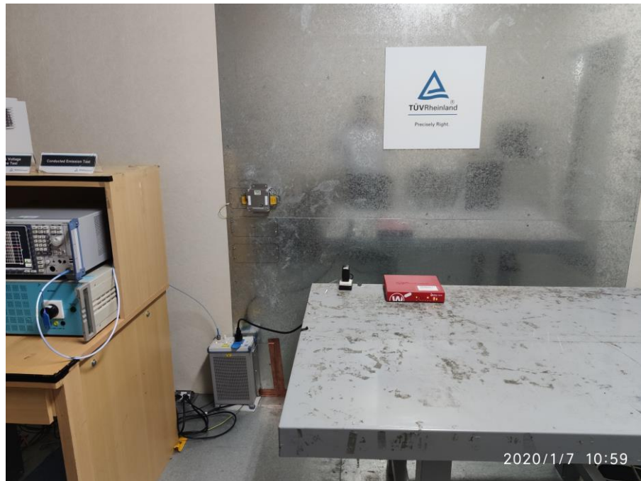
Photograph 6: Set-up for Mains Conducted testing (Front View)
